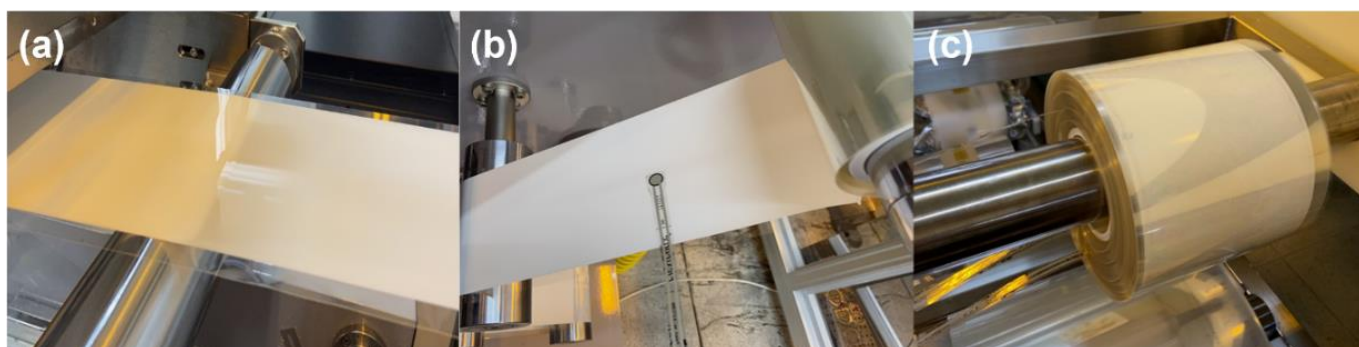
Figure 3. (a) Gadolinium-doped ceria coating layer; (b) the force-sensing resistor at the rewinding section; and (c) wound coated layer aging procedure.
