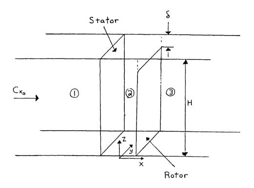
Fig. 2.1 Channel flow with constant blade-tip clearance
