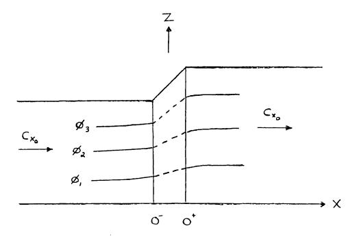
Fig. 2.5 Channel flow for variable density case
