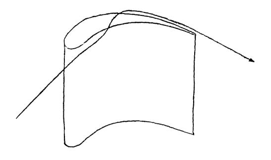
Fig. 2.6 Gap fluid that does some work on the rotor
