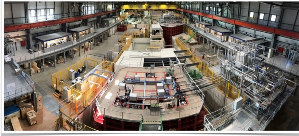
Figure 1.9. ProtoDUNE-SP and ProtoDUNE-DP cryostats in the CERN Neutrino Platform in CERN's North Area.
