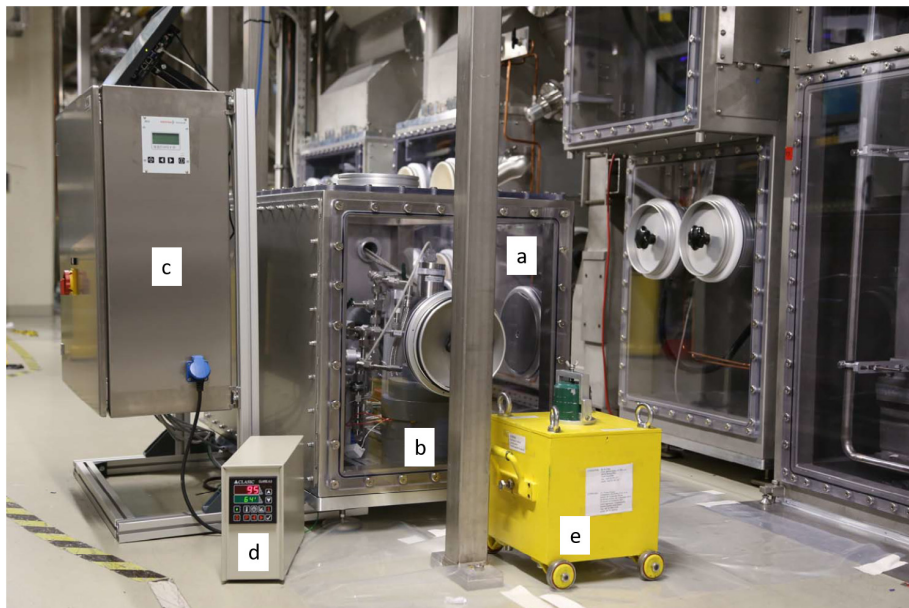
Figure 70. The ^{83m}\text{Kr} generator and transport container of the ^{83}\text{Rb}/^{83m}\text{Kr} zeolite source. Shown here are: (a) secondary containment with the generator (b) installed inside, (c) power distribution cabinet, (d) oven controller, and (e) transport container.
