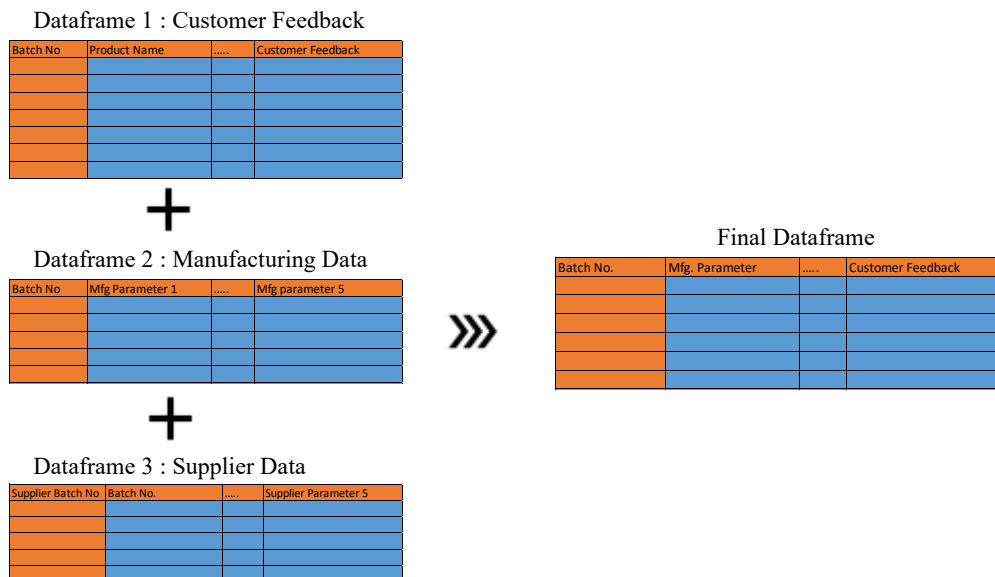
Figure 18: Dataframes merged to create final data table (Note that these tables are merged using a common identifier, Batch No. in this case.)
