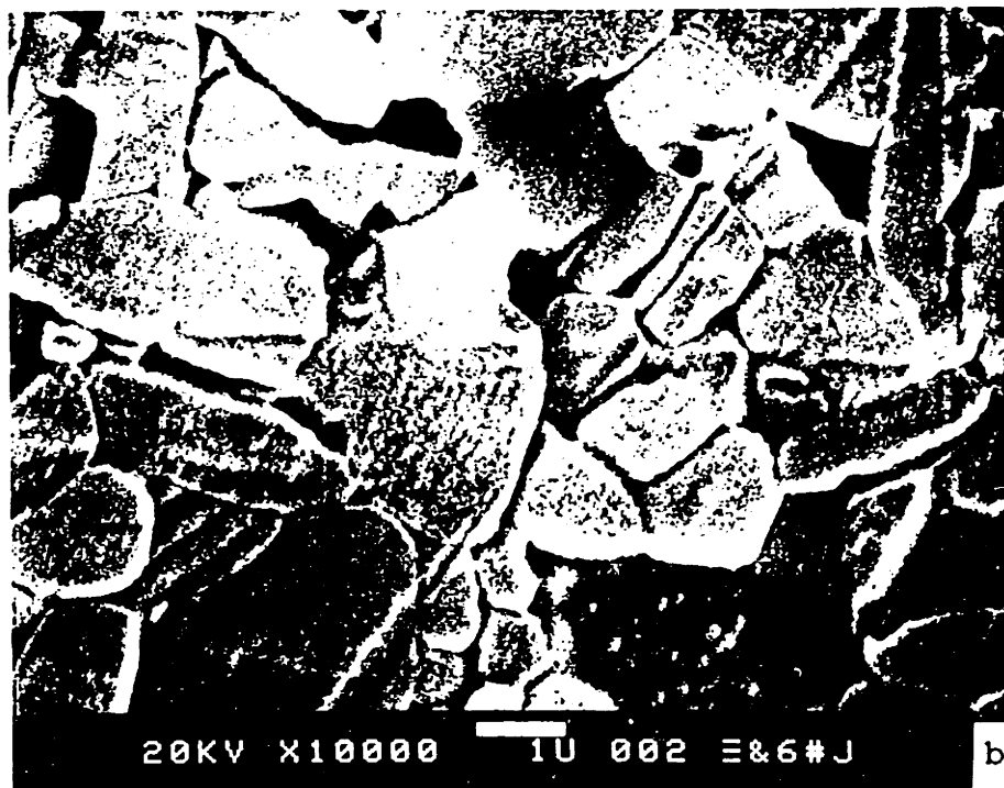
Fig.16. Polished and etched sections of samples "T7" (a), "T5" (b). ("T7": 6W% Al 2 O 3 , 2100 °C, 5h, packed in "T", semi-open) ("T5": 6W% Al 2 O 3 , 1950 °C, 5h, packed in 10-7, semi-open)
