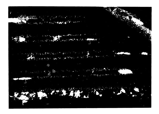
Figure 6 Dark field transmission electron micrograph (using the (110) vanadium and (1121) VSi<sub>2</sub> diffraction rings) of a vanadium/amorphous-silicon multilayer film which has been heated at 20 K/min to 808 K and quenched to room temperature; (a) polycrystalline vanadium; (b) amorphous-vanadium-silicide; (c) VSi<sub>2</sub> which has formed into a continuous layer (marked by arrows) between the amorphous-silicon and amorphous-vanadium-silicide; (d) amorphous-silicon.
