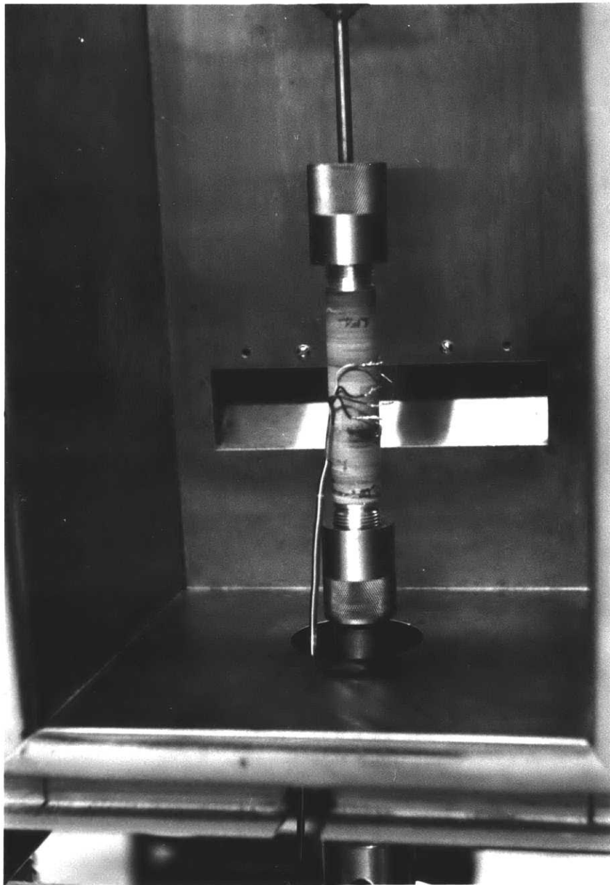
Figure II-1: Tensile specimen, grips and attached strain gages prior to heat-up and testing in the environmental chamber.
