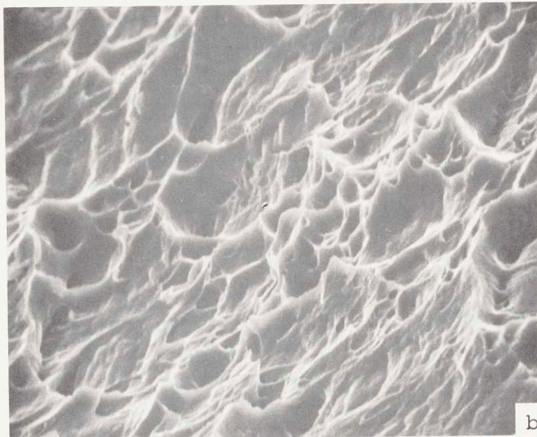
Figure 23: SEM fractographs of 99.5% aluminum. (a) As-received metal, 825X. (b) Filtered metal, 1120X.
