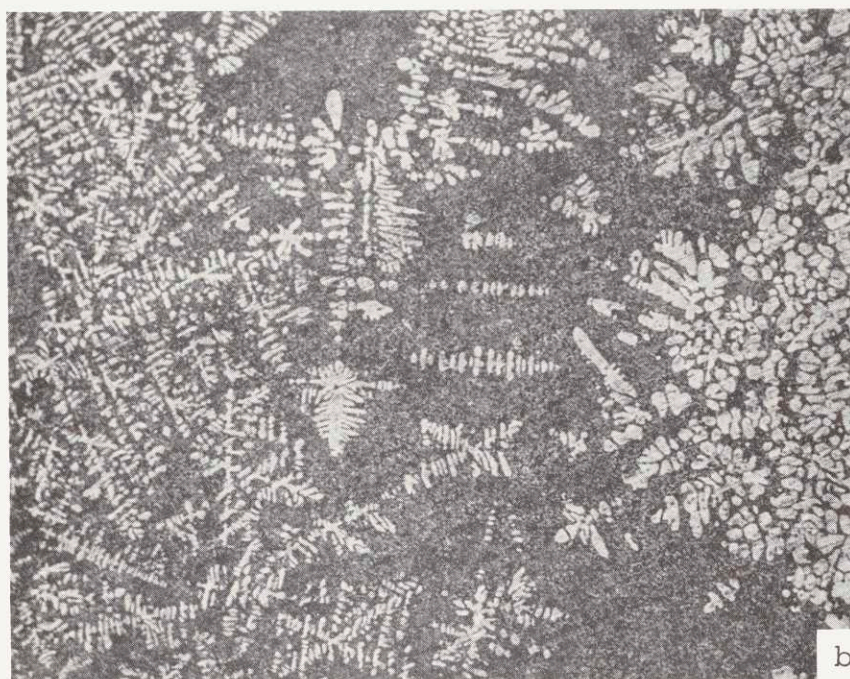
Figure 40: Structure of removed interdendritic liquid. (a) From Run #92, Al-4% Si-0.25% Ti alloy, 100X. (b) From Run #94, Al-4% Si alloy, 100X.
