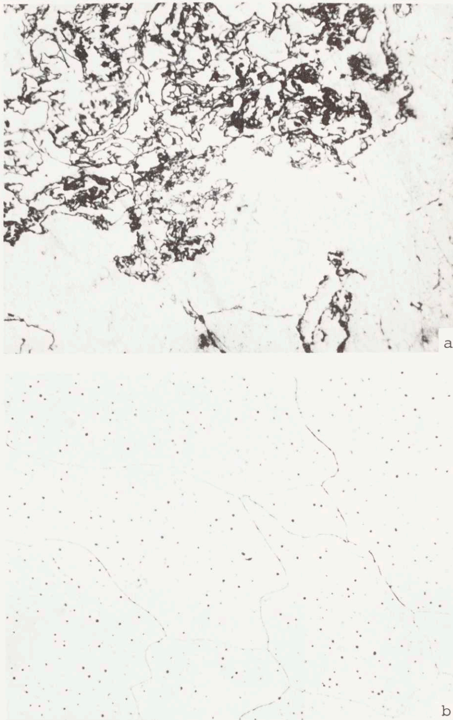
Figure 24: Microstructure of remelted granular aluminum before and after filtration, Run #51, Table IV. (a) Microstructure of metal immediately above flux coated \text{Al}_2\text{O}_3 granular bed, 75X. (b) Microstructure of filtered metal, 80X.
