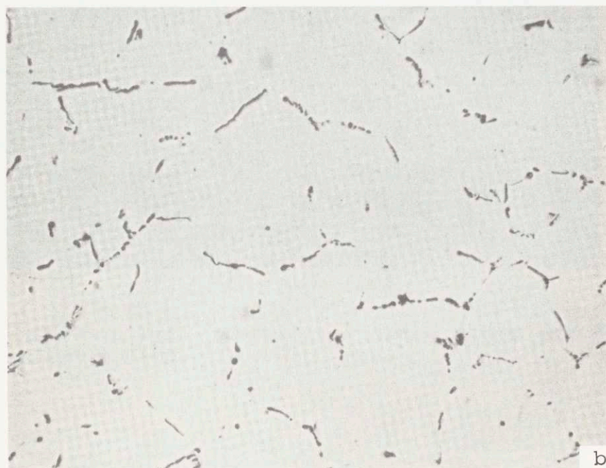
Figure 19: Microstructure of filtered and non-filtered metal in Run #12A, employing 216\mu Al_2O_3 granules followed by a sintered Al_2O_3 disc filter of 40\mu pore size.
