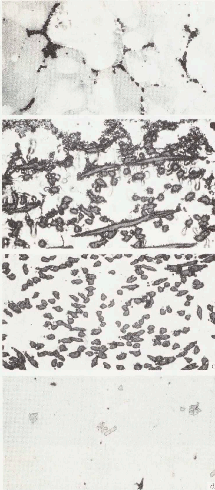
Figure 36: Microstructure of metal from Run #44b. (a) Metal above cake, 200X. (b) Entry port of filter, 200X. (c) Exit port of filter, 200X. (d) Filtered metal, 200X.
