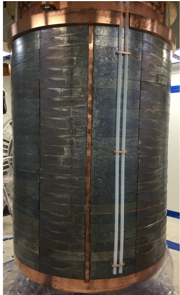
Extended Data Figure 2. Roman lead. Top left: the lead bricks recovery from the Sardinian sea. Bottom left: the ingot inscriptions were cut and preserved, while the ingot bodies were used for the CUORE internal lead shield 21 . Right: Lateral view of the internal lead shield 21 .
