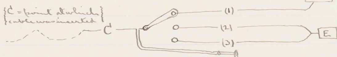
arranged so that by shifting a three-point switch I could ground the line at will through (1) a magneto generator, (2) a Blake instrument or (3) the loud speaker.
