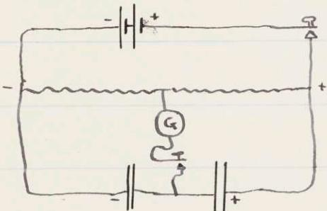
These are the connections for Scott's method. The equation is  $F_2 = \frac{R_1}{R_2} F_1$
