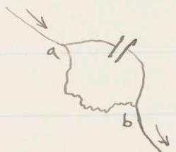
figure, the resistance ab was being measured and a condenser in shunt circuit kept absorbing electricity it would diminish the apparent resistance of ab. The battery circuit was kept closed long enough to get rid of any ordinary absorptive effect and moreover I believed the difference was of too great magnitude to be explained in this way.
