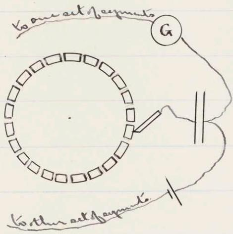
Have the other terminals of both connected to same terminal of condenser and the other terminal of condenser to a brush rubbing against perimeter of wheel. The rotation of wheel would effect the desired object. The condenser would be alternately charged and discharged and by varying the velocity of rotation of the wheel this could be made to occur any desired number of times per second.
