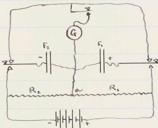
Annexed is a diagram of connections for the former method. The equation is  $F_2 = \frac{R_1}{R_2} F_1$ .
