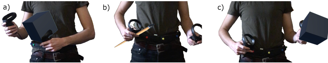
Figure 3-1: a) Pushing a button while holding a virtual object assigns the object to a Pocket. b) Different objects can be assigned to each Pocket. c) Objects can be retrieved by pushing the corresponding button. Because Pockets use physical hardware, and because we return objects to the dominant hand, we do not need to track their location.
