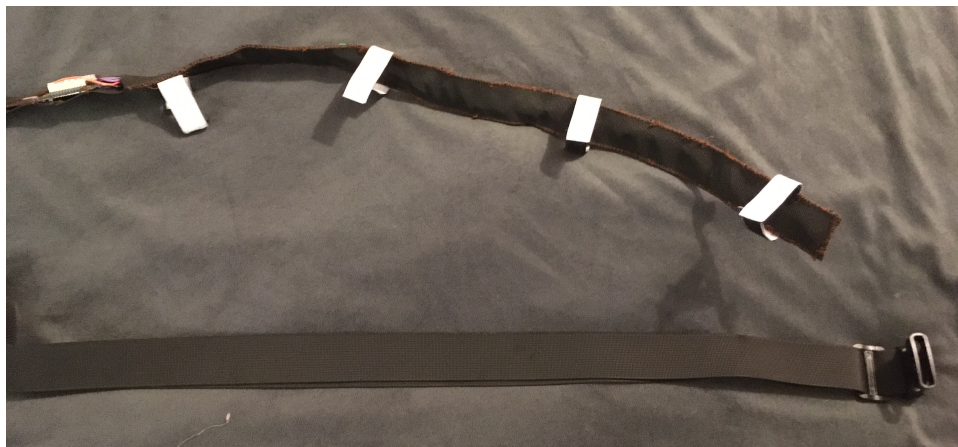
Figure 3-5: The tool belt separates into two parts, held together with Velcro straps. This allows the belt to be extremely adjustable, but the buttons to be a fixed distance apart.
