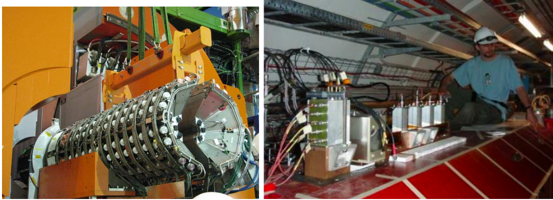
Figure 3-15: The picture of the CASTOR (left) at the CMS underground collision hall and ZDC (right) at 140 m away from the CMS beam interacting point are shown above.
