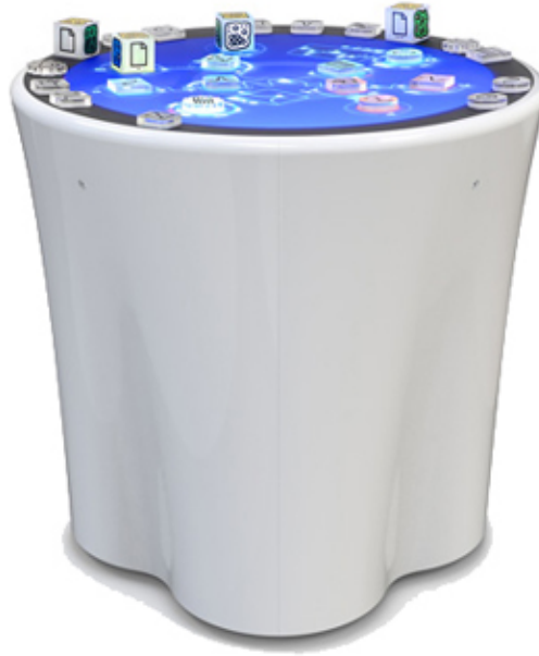
Figure 6: The installation version of the Reactable, showing the display screen on the table's surface, with several sound blocks placed on and off the controller. 15
