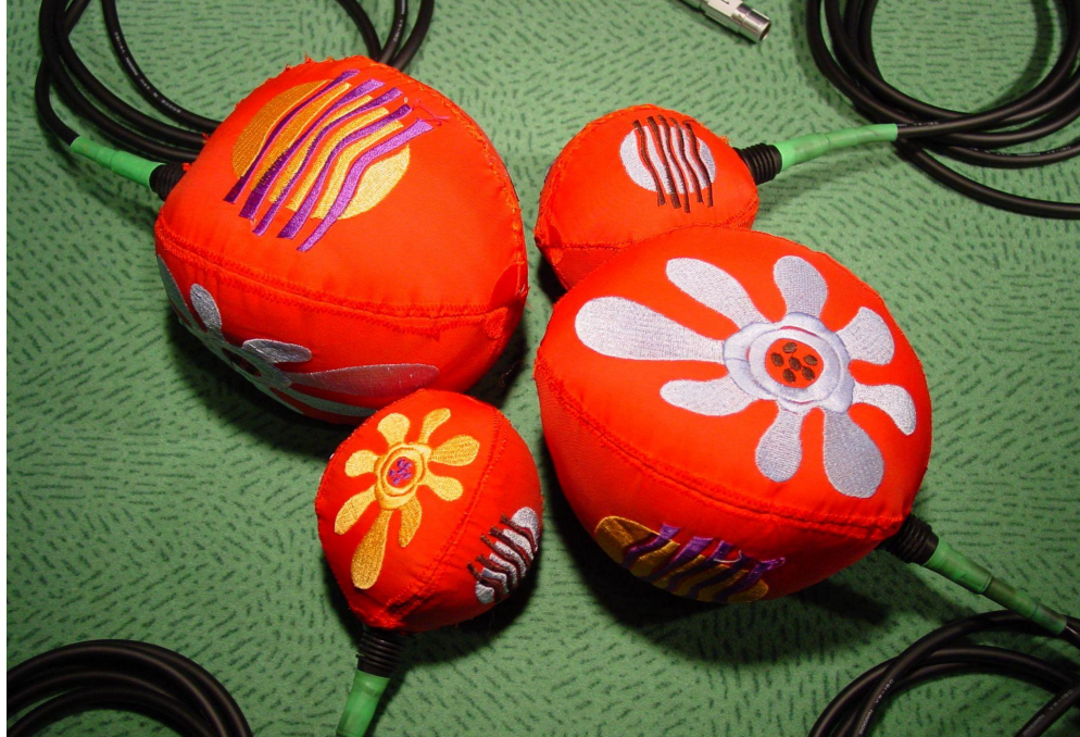
Figure 3: Four of the Music Shapers, displaying the different patterns of conductive embroidery. These were the instruments used in Tod Machover's Toy Symphony . 12
