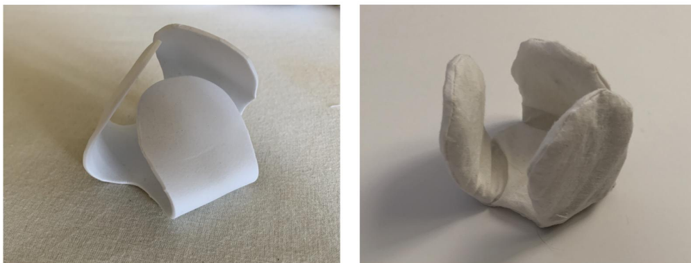
Figure 29: Craft foam shaped with a heat gun, and the same foam inserted into a fabric shell.
