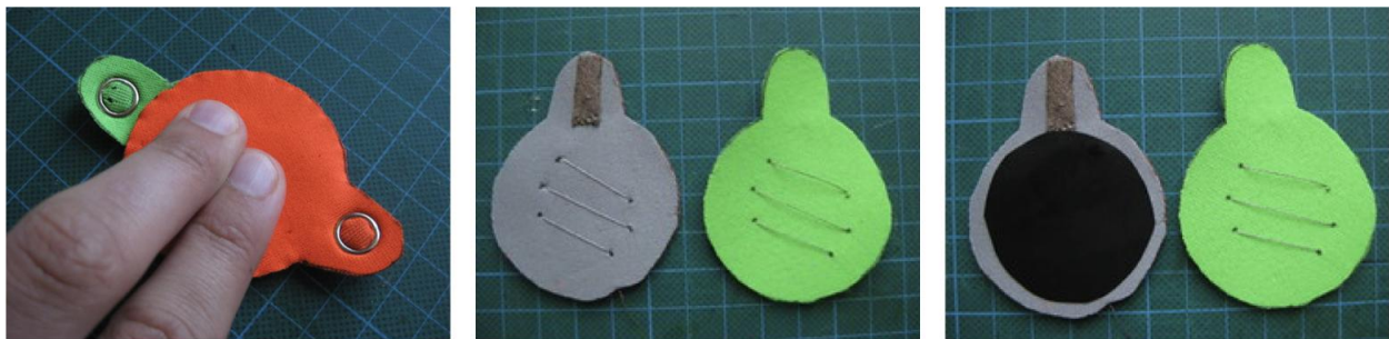
Figure 15: A fabric pressure sensor breakdown, created by Hannah Perner-Wilson for Kobakant. 27
