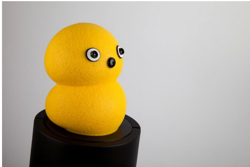
Figure 17: The MyKeepon robot, which will dance to music by bouncing up, down, and side to side. 29
