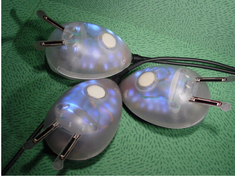
Figure 4: Three Beatbugs with translucent outer shells that show where a user can input percussive beats on the body, and where they can shape the sound they create, with the antennae. 13
