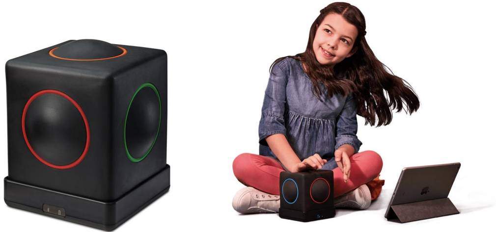
Figure 8: The Skoog instrument, shown with a user interacting with it - the circles on each side represent the sensitive areas. 17
