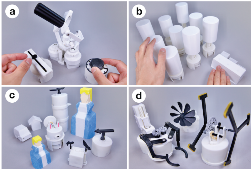
Figure 5-5: Overview of interaction design purposes and benefits of Mechanical Shells from instances of HERMITS (a. Tangible and Haptic Controllers, b. Data Physicalization / Tangible Representation, c. Storytelling with Expressive Shapes and Motion, and d. Extended Robotic Manipulator and Locomotion)
