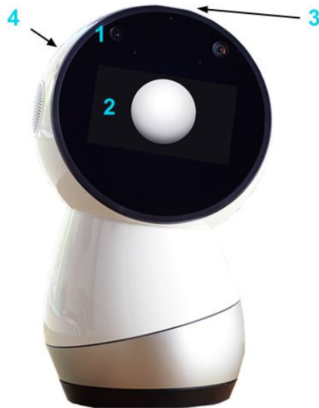
Figure 4-1: A photo of the Jibo robot. Jibo has cameras (1), a touch screen (2), a touch sensor (3), and microphones (4).
