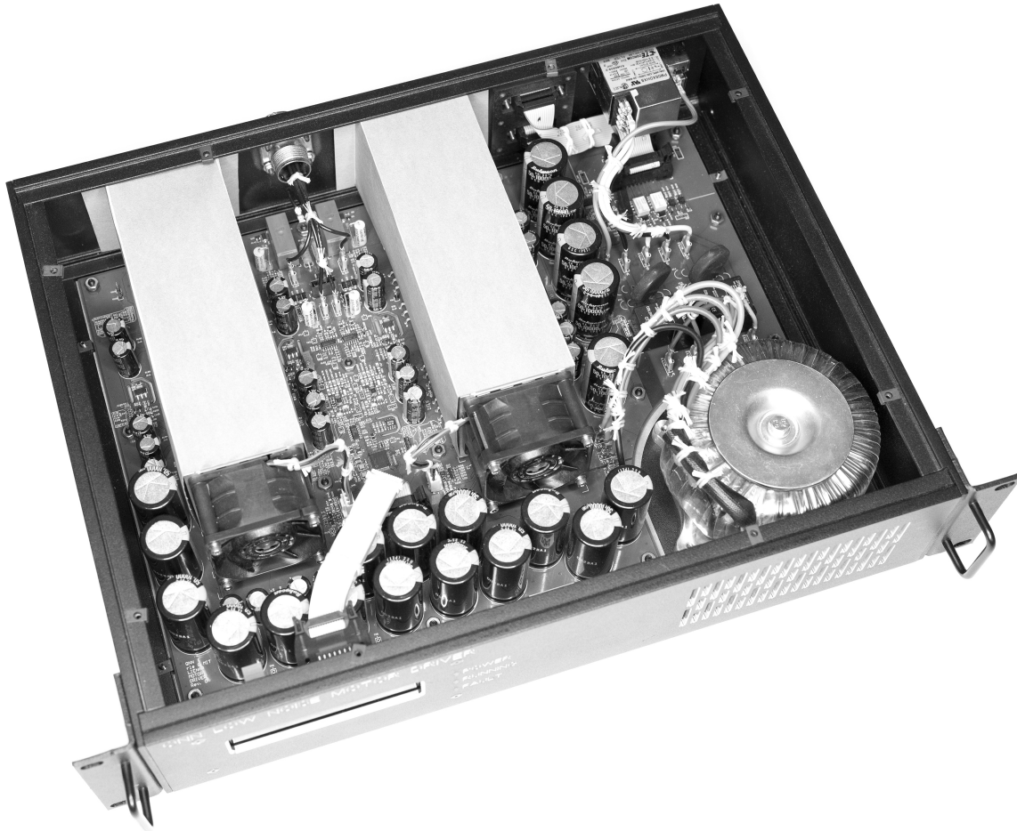
Figure 5-5: Photograph of the linear motor driver with the top cover removed. The unit consists of a 2U 19" rack-mounted enclosure. The device status and configuration is shown by three LEDs and an LCD screen on the left of the front panel. On the right of the front panel is the air intake, and the exhaust is at the back of the unit. The power input module (power connector, fuse, and voltage selection switch) is mounted on the back panel. An isolated panel houses the serial port and interface port. Finally, a circular connector on the back panel connects to the motor.
