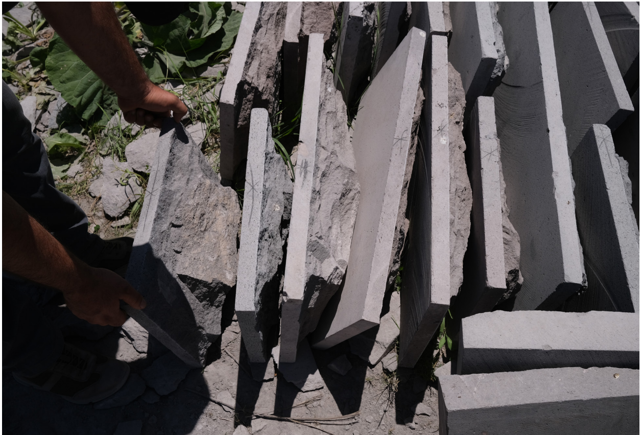
Stone with polished facing (սրբասուաշ) and rough-cut backing (կոպսասուաշ). Used for “midis” technique of construction.
