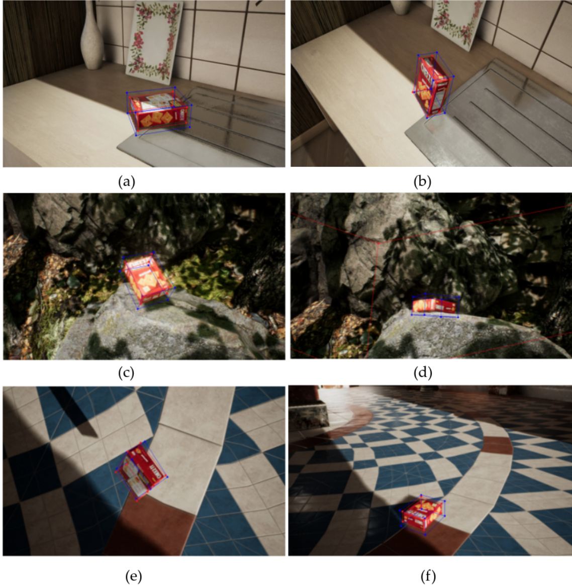
Figure 5-5: Ellipsoid estimates from VoluMon Primal Only visualized as blue bounding boxes, and the estimates from DOPE visualized as red bounding boxes using the ground-truth object size. VoluMon constrains the projected centroid of the object to fall within the 2D object bounding box, helping to avoid some failure cases of DOPE, e.g., top row, right column. Additionally, while VoluMon tends to slightly overestimate the size of the object, many of the estimates appear qualitatively reasonable.
