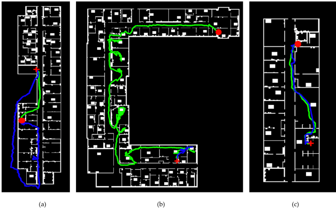
Figure 3-10: Comparative examples of planning performance, where the robot begins inside and is given the contextual information that the goal is also indoors (II). We show the final trajectories of the learned (green) and baseline (blue) planners traversing from start (red cross) to goal (red circle). In (a), the baseline planner mistakenly exits the building although the goal is indoors, but the learned planner largely remains in hallways and reaches the goal. In (b), the baseline planner fails to find a trajectory with the allotted sample count, while the learned planner mistakenly visits many rooms. Such a case is not included in the aggregate metrics as the baseline planner failed. In (c), both the learned and baseline planners mistakenly enter rooms prior to reaching the goal.
