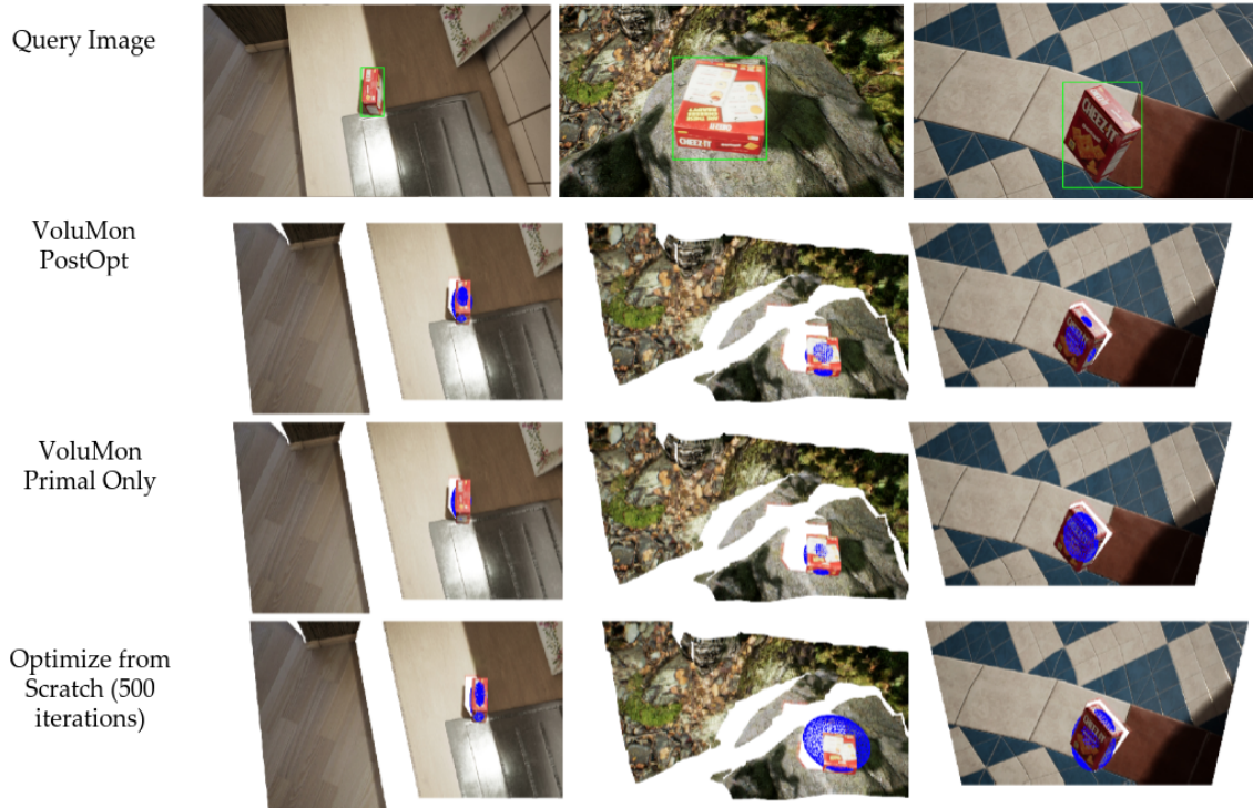
Figure 5-4: Qualitative results for selected methods. Ellipsoid estimates visualized as blue meshes. Although VoluMon PostOpt requires less steps of online optimization compared to Optimize from scratch (100 iterations), the initial pose estimates provided by VoluMon Primal Only enable VoluMon PostOpt to generate more accurate estimates of the ellipsoids. Potentially due to shape ambiguities, it can be difficult to estimate the extents of the object; by keeping the size estimate from VoluMon Primal Only , VoluMon PostOpt benefits from observations over a dataset to estimate size at run-time.
