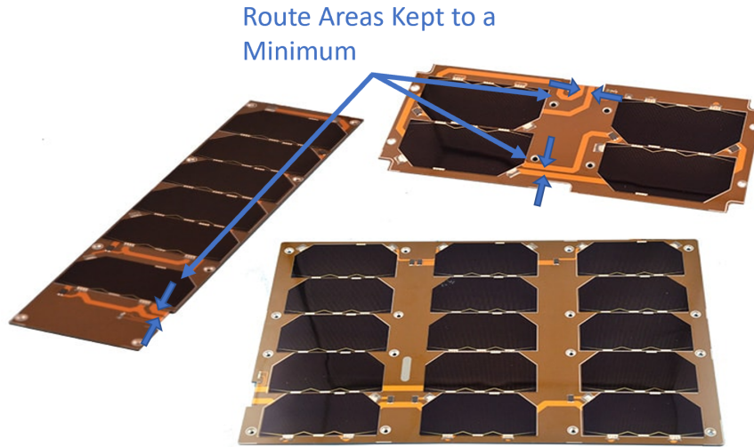
Figure 2-11: ISIS solar panel arrays have been routed for minimum current path loop area [3]. This reduces radio frequency EMI and minimizes the perturbing magnetic field.
