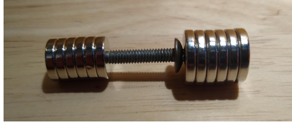
Figure 6-6: Using neodymium magnets to magnetize an object of unknown material.
