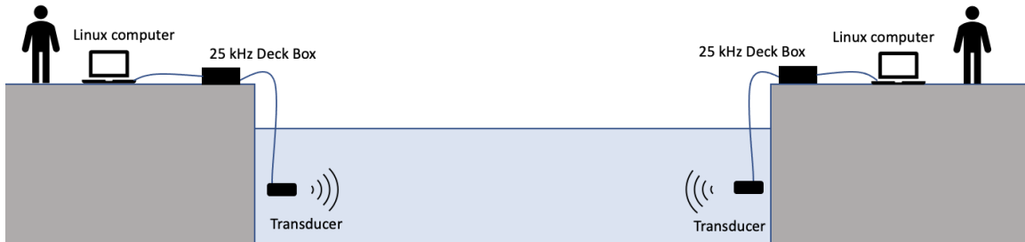
Figure 4-2: Static ping test set-up.
