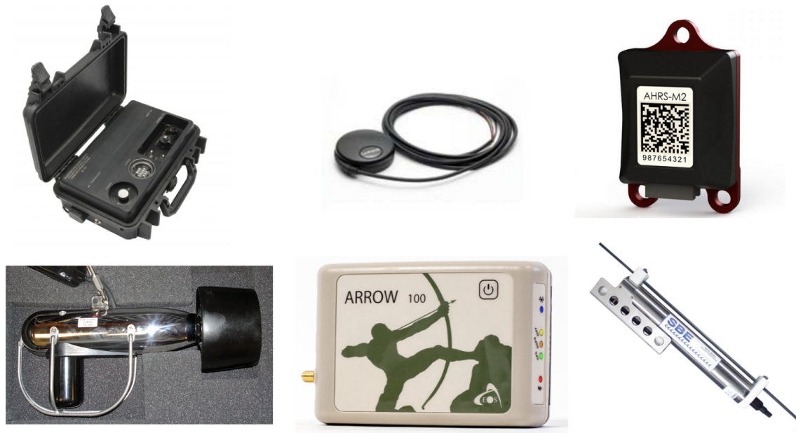
Figure 4-1: Key equipment used during our tests and experiments. Top left: Micromodem 2 25-kilohertz PSK deck box [82]. Top center: Garmin GPS 18x receiver [84]. Top right: Sparton M2 AHRS [74]. Bottom left: 25-kilohertz transducer towfish [50]. Bottom center: Arrow 100 GNSS receiver [83]. Bottom right: Sea-Bird Scientific SBE 37 SMP pumped MicroCAT [85].
