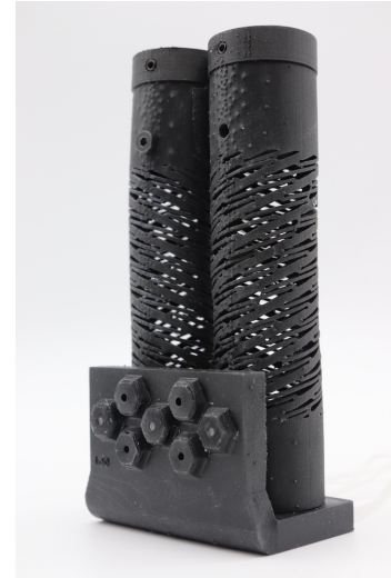
Figure 6-3: Left: Evaluation of 3 tactile sensors on one tactile sensor array against increasing applied load. The three outputs from one array are averaged to give a single measured output in millivolts. Standard deviation is also shown. Right: Hardware setup with digitally-fabricated HSA fingers and digitally-fabricated hexagonal tactile sensors.
