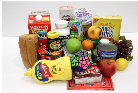
Figure 6-1: 25 hand-labeled calibration items were evaluated to determine the priority packing heuristic. Soft: clementine, grapes, juice box, mozzarella cheese. Medium: book, celery salt, empty soda can, instant ramen, jello, milk carton, mustard bottle, toy peach, toy pear, wheat thins. Rigid: apple, coffee can, fake cake, plastic lemon, Pringles tube, Rubik's dodecahedron, Spam, tea box, tuna can, vegemite, vitamin bottle.
