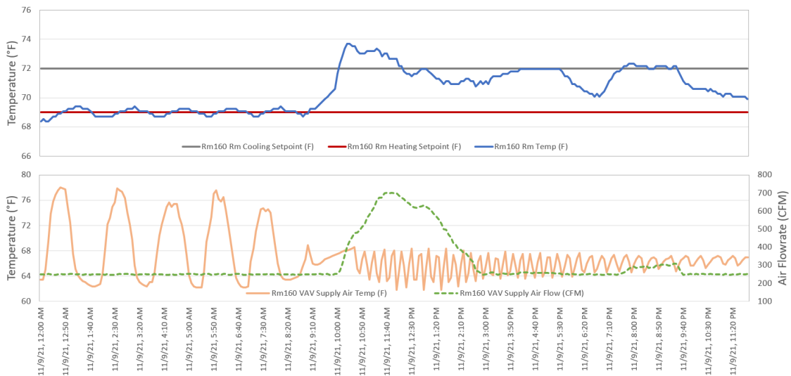
Figure 7-3: [Room 160] Setpoints, room temperature (top), VAV supply air temperature and supply air flowrates (bottom) on Nov. 9
