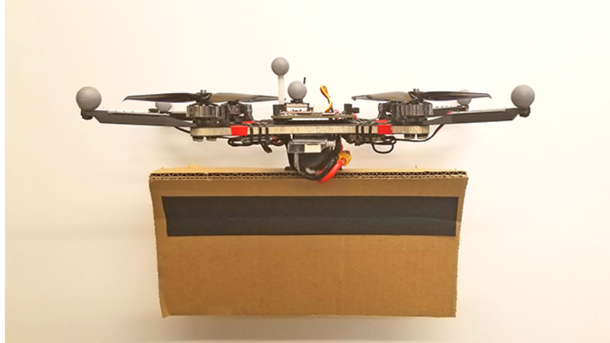
Figure 2-14: Quadrotor with 16 cm \times 32 cm cardboard drag plate.
