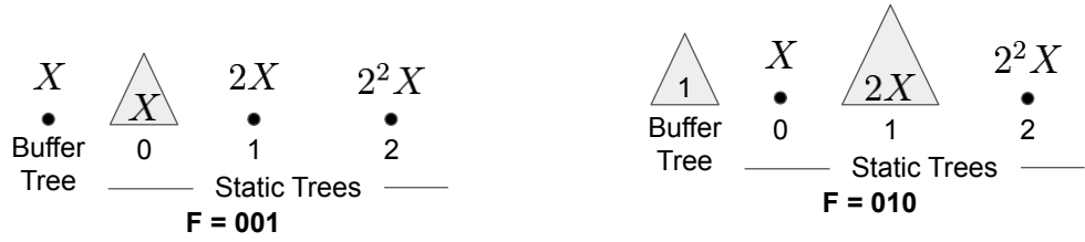
(b) Static tree 1 is full and buffer tree has 1 point.
