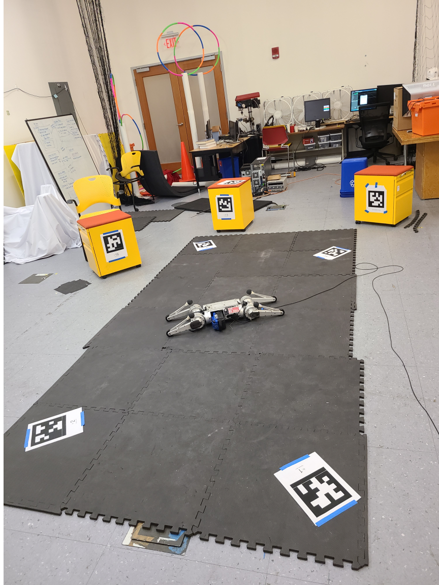
Figure 4-1: Experimental set up for final test, moving trot. There were three April-Tags on rolling drawers, and four on the ground. The cheetah did two laps of the course for the test.
