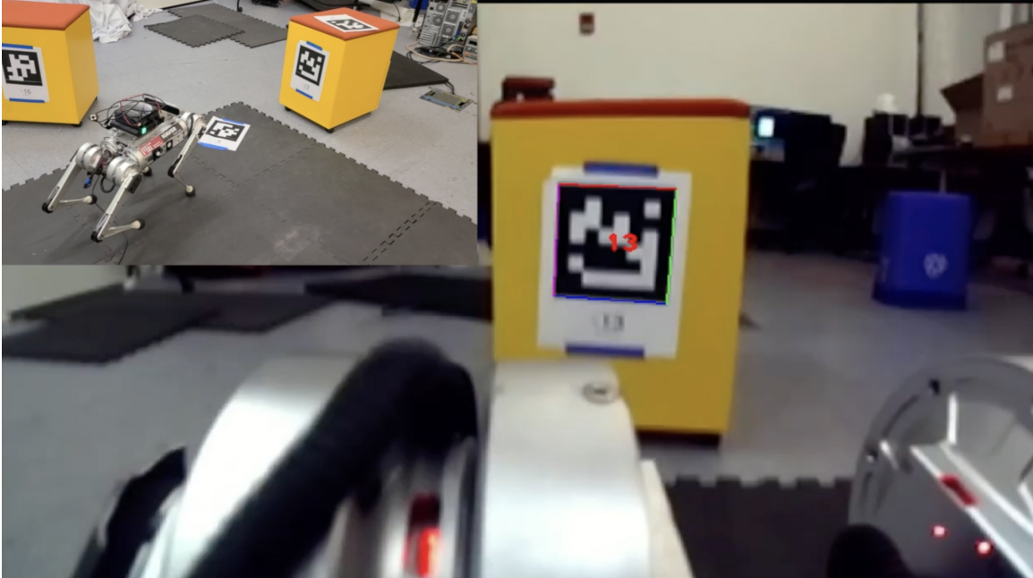
Figure 5-3: Visual data of rigidly mounted camera with stationary pronking. The AprilTag was detected throughout most of the test, even with the pronking gait. The video can be accessed here .
