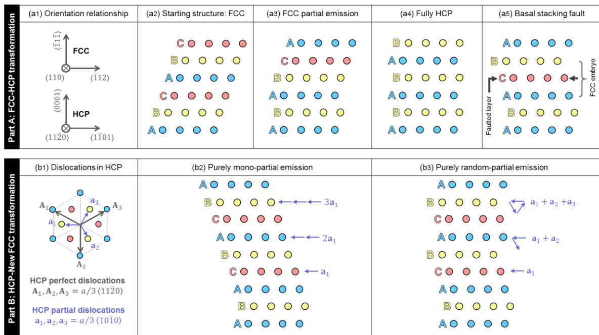
Figure 3.8: Atomistic processes for the sequential FCC-HCP-FCC transformation. (a1)-(a5) the FCC-HCP transformation; (b1)-(b3) the HCP-(new)FCC transformation.
