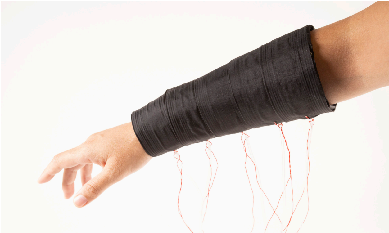
FIG II. 11 Final prototype of the pneumatic Affective Sleeve. Side view of the fastened prototype. The outer view of the prototype remains the same in both inflated and not inflated states.
