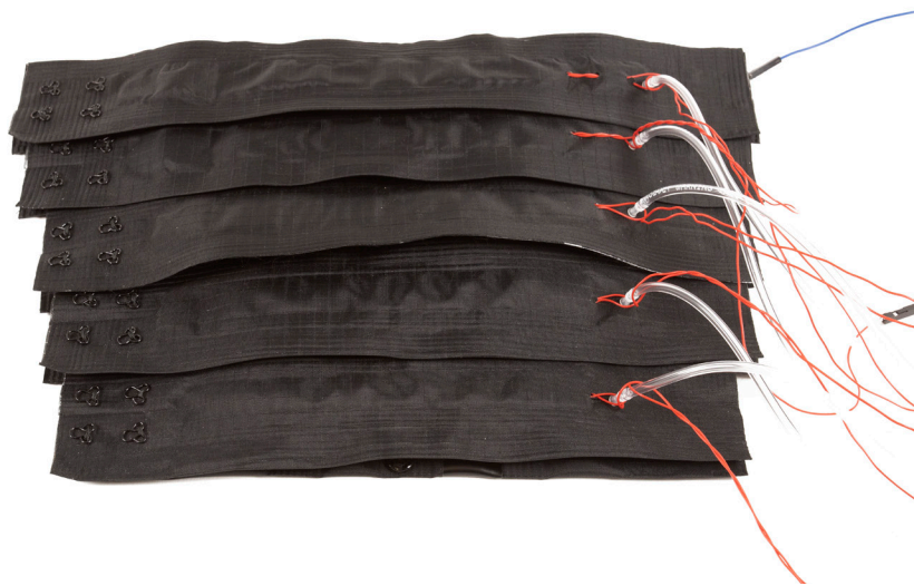
FIG II. 10 Final prototype of the pneumatic Affective Sleeve. View of the unfastened prototype showing how the cuffs overlap with one another allowing both individual control and maximum coverage.
