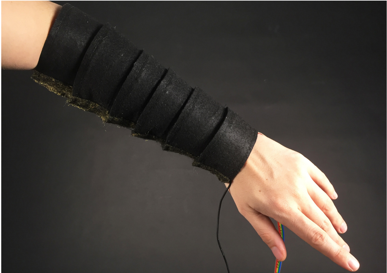
FIG I. 3 Final prototype of the Affective Sleeve made from felt fabric, nitinol wire and elastic bands. Top view
