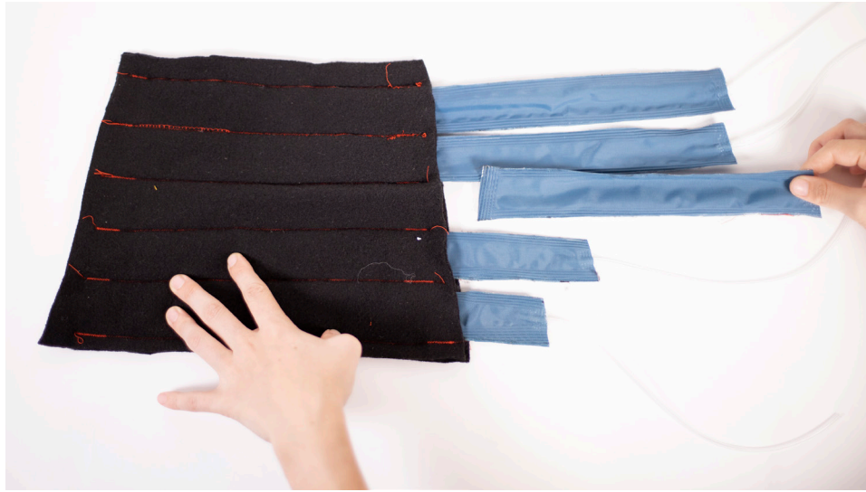
FIG II. 1 Early prototype of the pneumatic Affective Sleeve consisting of two layers of fleece fabric sewn together in six places, creating five compartments that act as pockets for the inflatable inserts. Top view of unfastened sleeve (top). Side view of the fastened sleeve (bottom)
