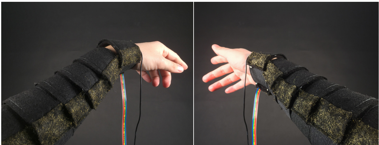
FIG I. 4 Final prototype of the Affective Sleeve made from felt fabric, nitinol wire and elastic bands. Side views
