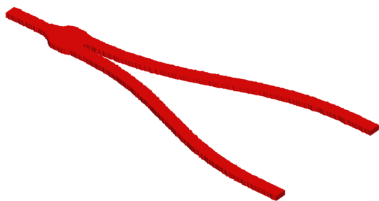
Figure 2-1: Line edge roughness imposed on a Y-branch and waveguide sidewalls.
