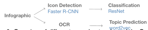
Figure 6: Overview of different neural network models. Our icon detector is used to locate icons, which are then classified into one of 391 tag categories using a separately-trained icon classifier. We simultaneously run a text detector and feed its output to a topic prediction module. Together, these models open new avenues for summarizing and parsing infographics as presented in our applications.
