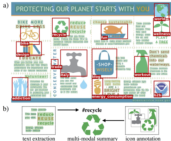
Figure 8: a) The output of our fully-automatic annotation system, running text detection and OCR [28] (semi-transparent green boxes), with our own icon detection and classification (red outlines). We trained an icon detector with synthetic data to make this system possible. The underlying infographic has been faded for visualization. b) Our multi-modal summarization application uses the detected text and icons to produce the text tags and visual hashtags most representative of the infographic’s topics. ©oceanservice.noaa.gov
