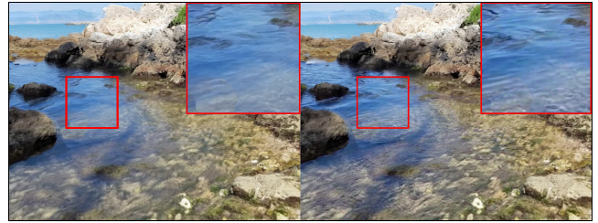
Figure 14: Results for the Seaside scene. Our per-frame improved version of ULR (left) [BBM*01] and our result (right). The low frequencies are reprojected onto the sea-floor while the high frequencies are reprojected onto the water plane, allowing correct parallax when moving the viewpoint.
