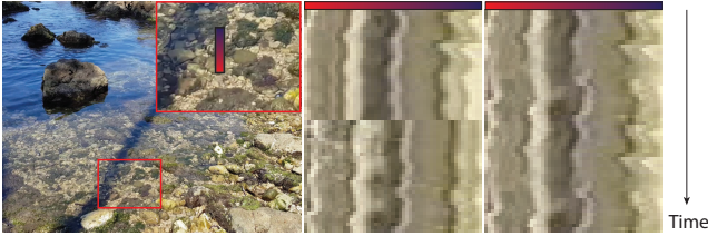
Figure 6: Video looping. Natural videos played back to back show a strong temporal discontinuity (middle), while our temporal Laplacian blending scheme produces a seamless video loop (right). Slices are represented with time on the vertical axis and space on the horizontal axis. Displayed slices correspond to the zoomed-in segment (left).
