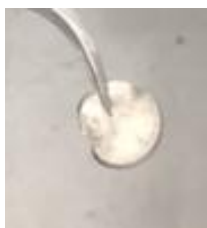
Figure S16: Photograph of Li metal anode post discharge with DIPA- \text{CO}_2 in 0.3 M \text{LiClO}_4/\text{TEGDME} at 70^\circ\text{C} .
