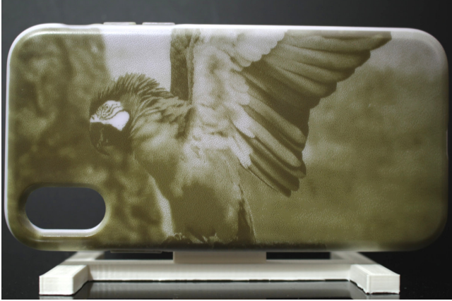
Figure 2: Grayscale preview: Physical result of projecting a dithered grayscale image onto a physical sample using only the UV projector.
