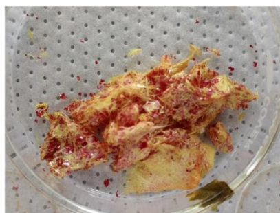
Figure 3-6. Picture of n = 2 BA-MAPbI crystals with yellow, needlelike crystal byproducts.
