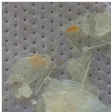
Figure 3-30. Orange coloring on white crystals of n = 1 BA-PbBr. Because the synthesis of n = 1 BA-PbBr does not involve MA cation, these orange colorings are not believed to be due to the formation of bulk MAPbBr 3 or higher members of bromide 2D LHPs.
