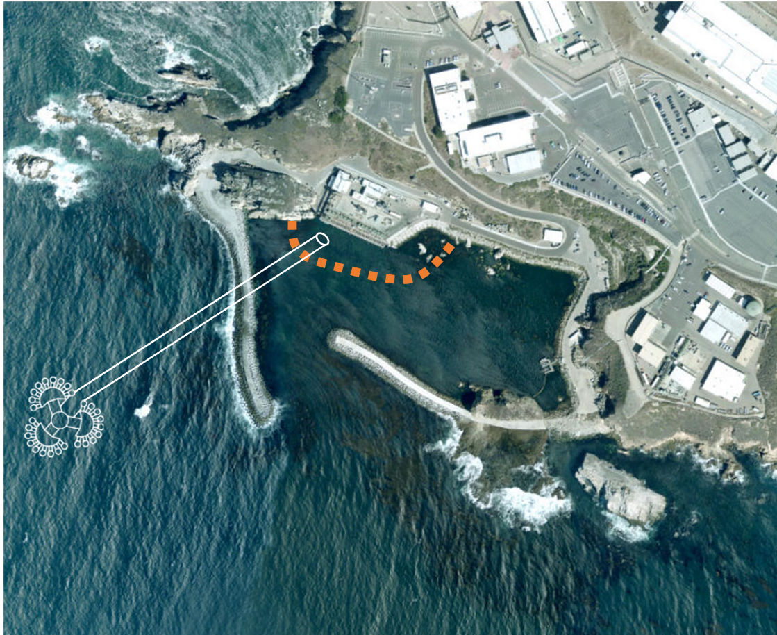
Figure 3: Aerial view of existing DCNPP intake lagoon with superimposed lines showing one possible approach to building a new intake structure. Dotted lines represent an additional impermeable basin with a tunnel extending offshore, connected to a wedgewire screen array for Options 1–3. Option 4 requires two additional tunnel and screen arrays. The new basin would have an emergency water inlet to ensure water flow to the reactors in case of blockages, damage, etc.
