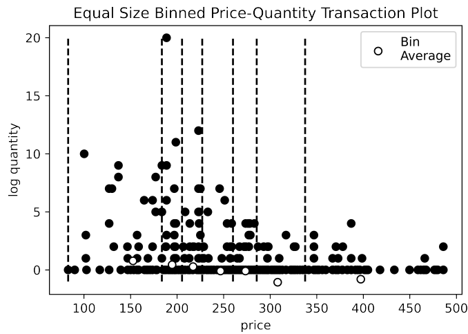
Figure 4-6: Graph depicting the transaction data from Figure 4-2, grouped into bins that each contain an equal number of points (in this case, m = 200 ). Each bin is created by taking the next 200 points (as ordered by price values) that have not yet been binned. The average of each bin is shown in the white dots on the chart. While still mostly close to zero (data is displayed on a log scale), this method helps to remove some outliers and assist with slightly better curve fitting.
