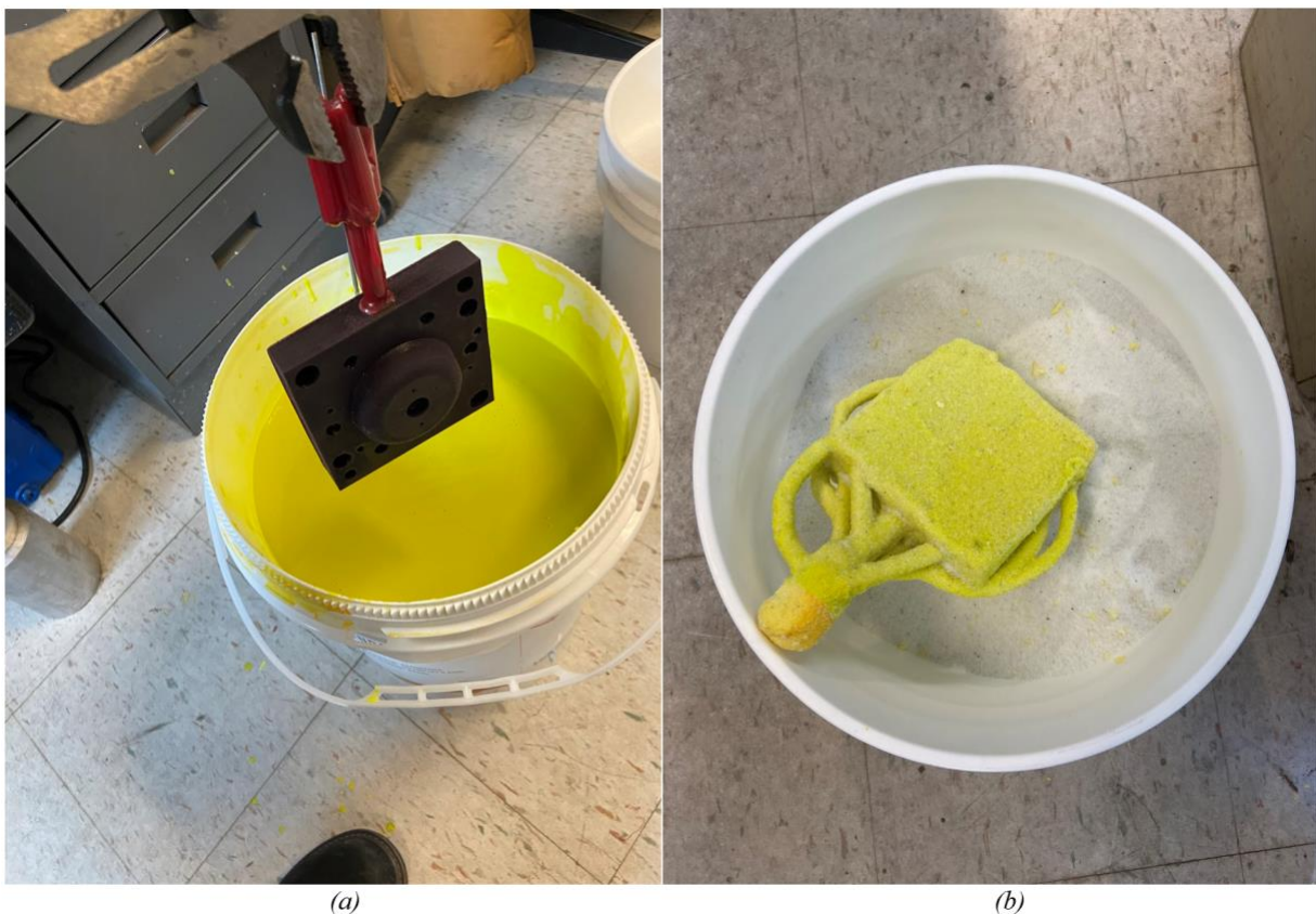
Figure 8: (a) A part about to be dipped in Suspendaslurry FS material, and (b) a part after being coated with Ranco-Sil B fused silica sand.
