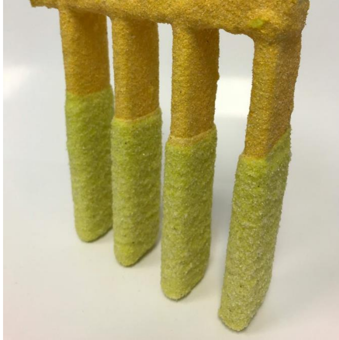
Figure 19: A comparison of dry Suspendaslurry material (the orange top half) vs. wet Suspendaslurry material (the yellow bottom half) [16].
