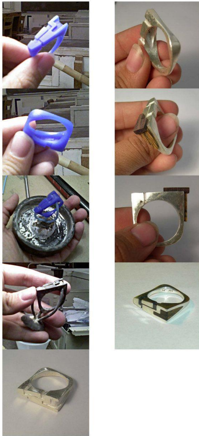
Figure 3: An investment cast ring at all steps of the investment casting process [9].
