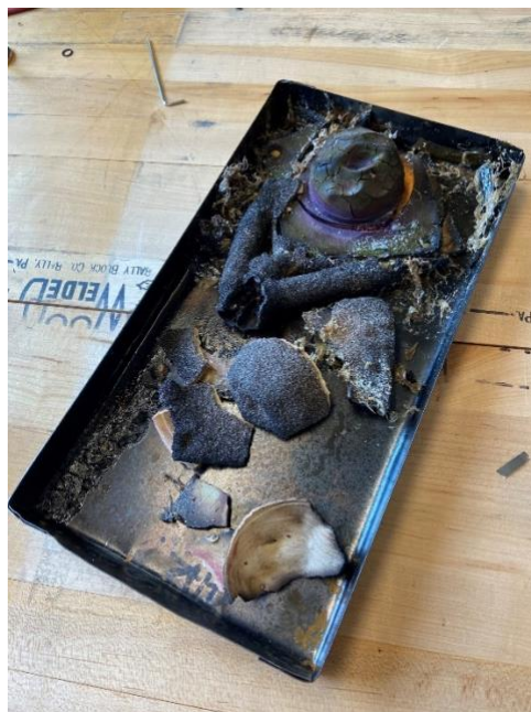
Figure 23: The remains of test part 2 after catching fire in the furnace. The ceramic shell was cracked open, revealing the intact 3D printed part still inside.
