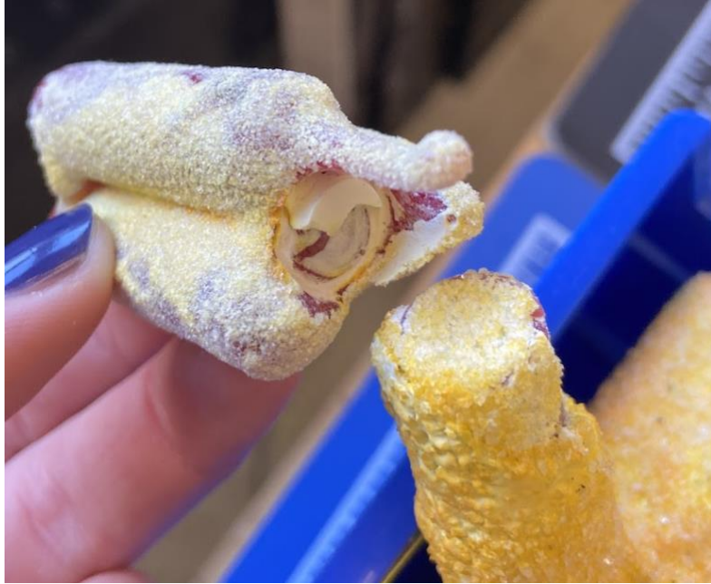
Figure 20: The broken sprue of part 1 that fell off while dipping.
