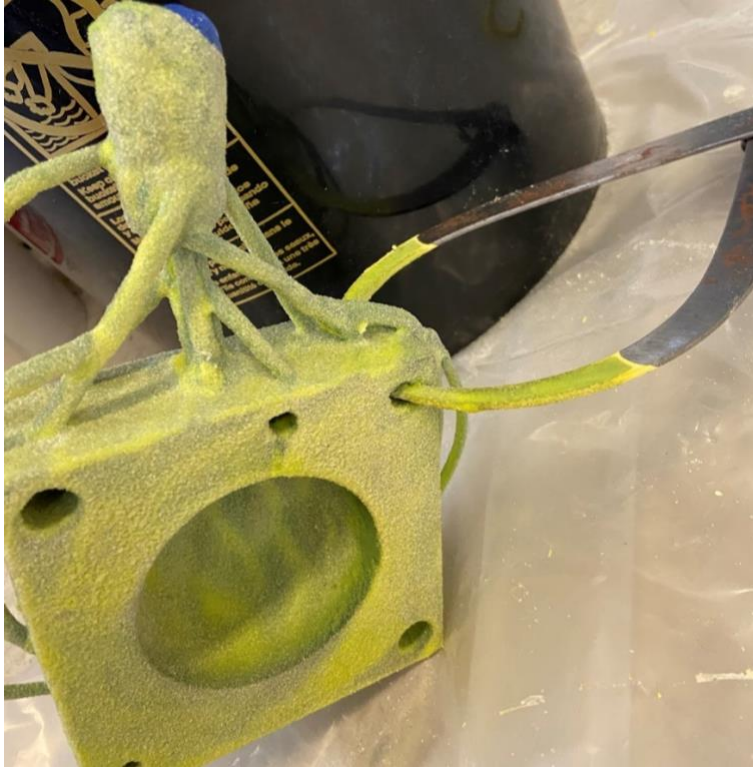
Figure 21: The holding configuration used while dipping part 3.
