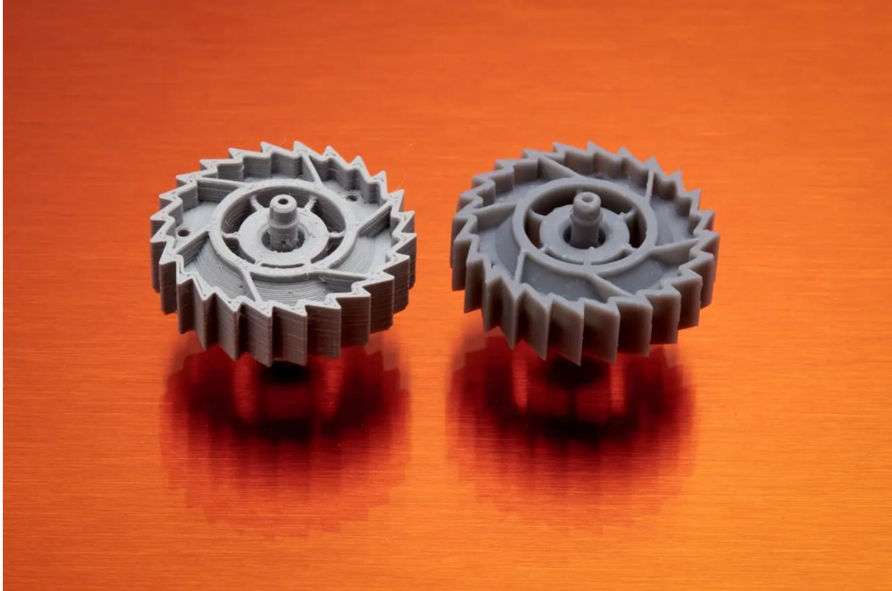
Figure 2: A comparison of an FDM printed part (left) and a SLA printed part (right). The SLA printed part has a much higher surface quality and is generally more durable, though it is often more brittle than FDM printed parts [5].
