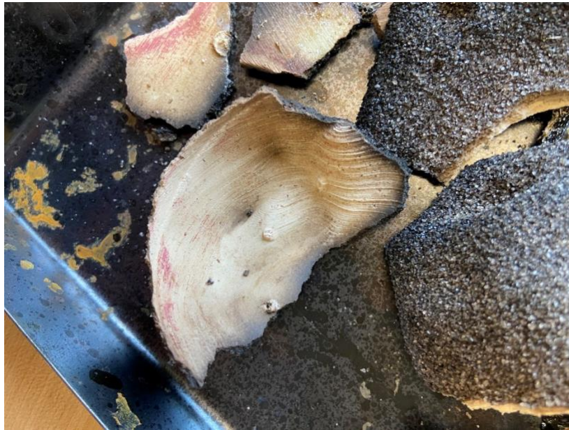
Figure 24: The inside of the cracked ceramic shell of test piece 2. The inner surface almost exactly matched the corresponding surface of the 3D printed part, indicating that the shell would have created a high quality cast part had it survived firing.
