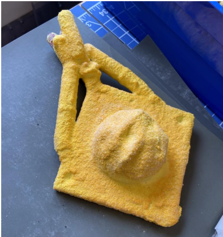
Figure 22: Test part 2 after being dipped and coated 4 times.
