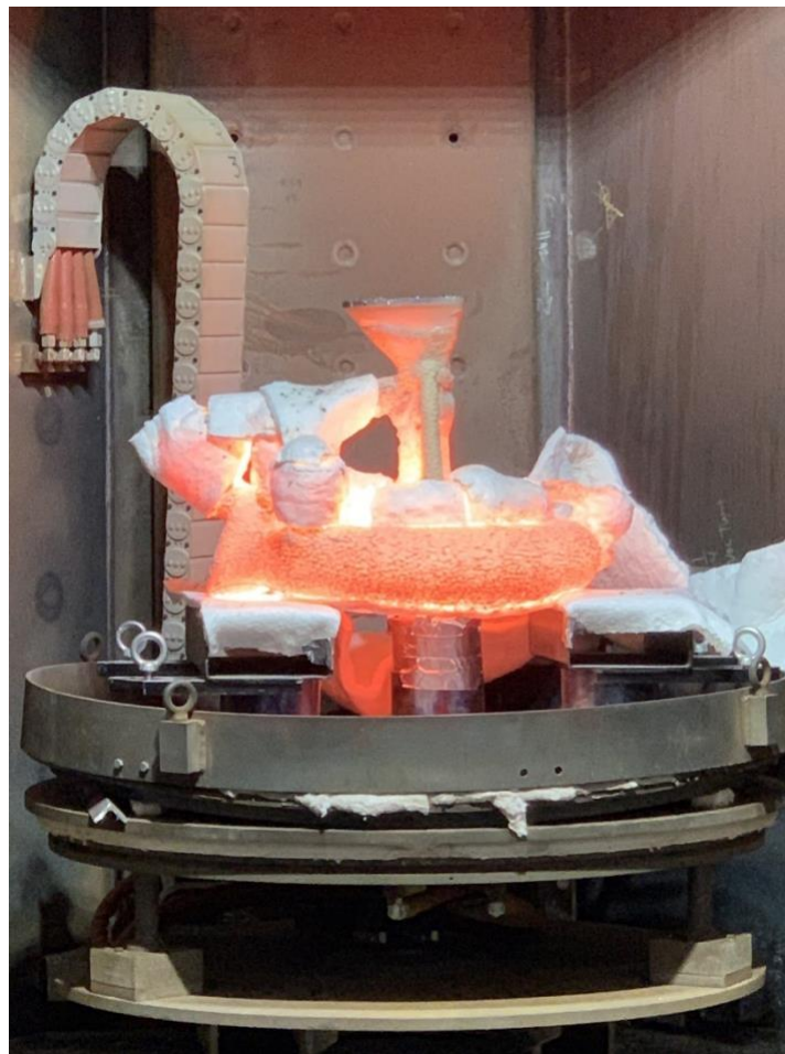
Figure 4: A recently poured Raptor manifold from the SpaceX Foundry [11].
