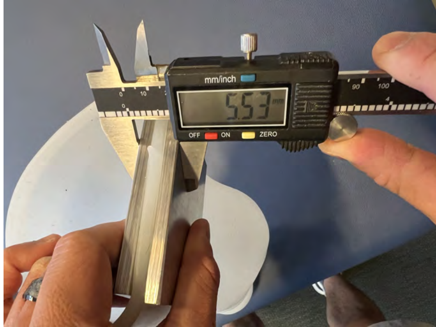
Figure 2-1 Liner Thickness Measurement Technique
