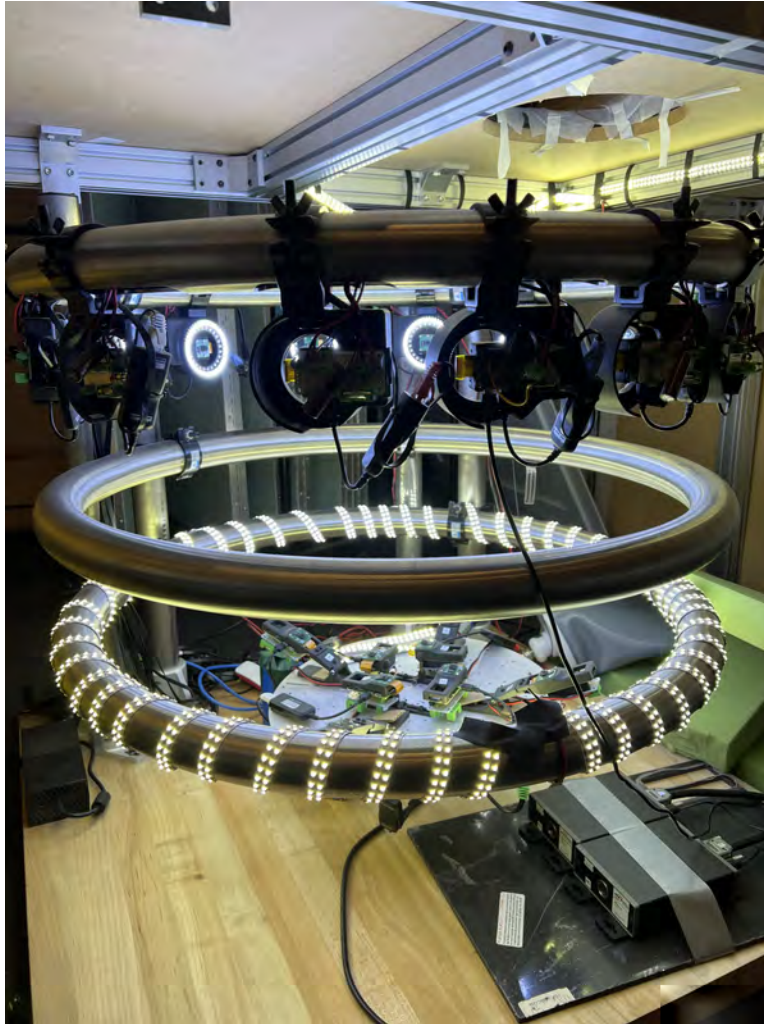
Figure 1-4 The digital image correlation system developed and used in Biomechanics.
