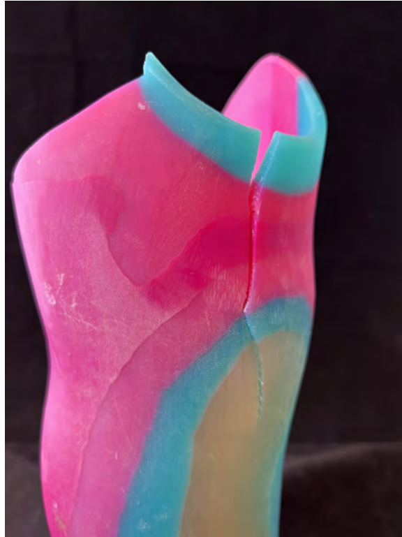
Figure 1-2 A crack in a multi-material socket that already lost the medial lobe due to material failure.
