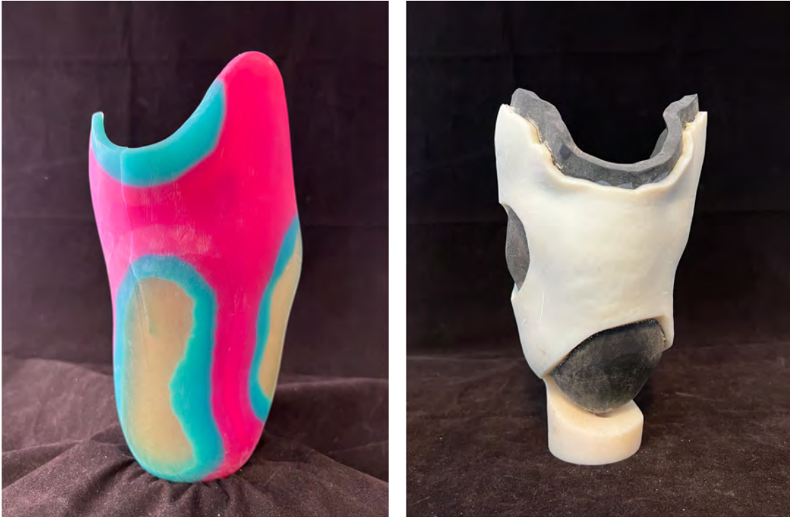
Figure 1-1 Two examples of multi-material sockets produced by the Biomechatronics group. They use different algorithms to determine areas of variable material compliance, and are both 3D-printed. The one on the right was the product of David Sengeh's Ph.D. thesis [13].
