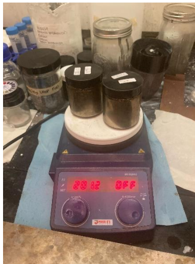
Figure 2 shows two jars of aluminum BBs undergoing the activation process
