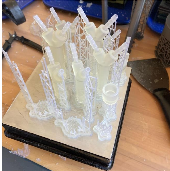
Figure 13 Build plate of 12 geometries printed at the same time using a high-temperature Formlabs resin
