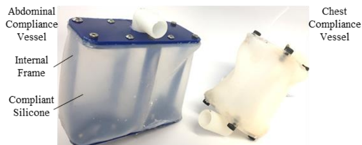
Figure 13: Compliance vessels. On the left, the abdominal compliance vessels and on the right, one of the two chest compliance vessels.
