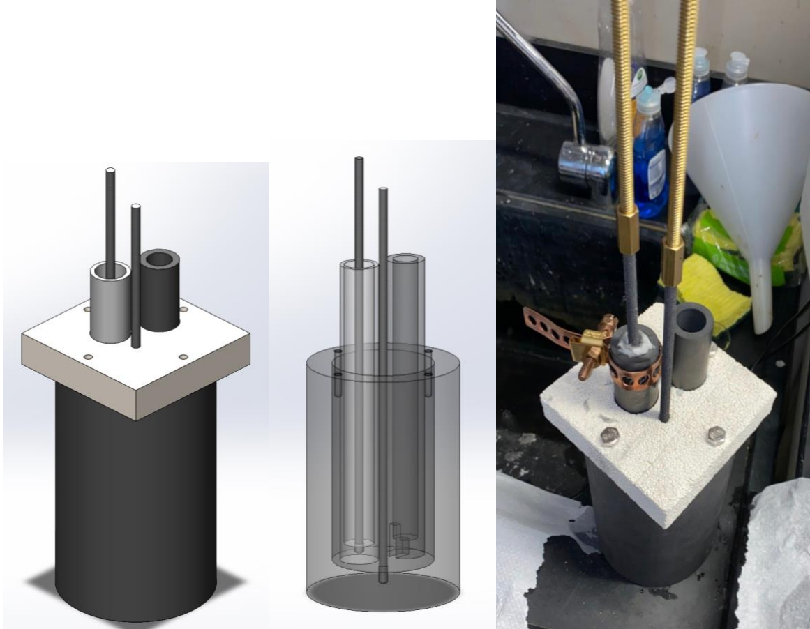
Figure 25: Rod-Sheath Height Measurement Prototype
