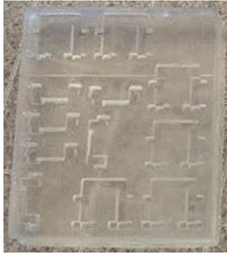
Figure 5.2: Mold for PDMS skeletons.
