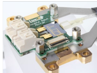
Figure 4-3: Examples of packaged tunable lasers produced by commercial entities Freedom Photonics and Lionix. A minimum optical power of 100 mW and a maximum line width of 240 kHz is required for 200 m ranging. The wavelength-based scanning in the vertical direction requires a tuning range of 100-160 nm. Adapted from Freedom Photonics [61] © 2022. Adapted from Epping et al. [62] © 2019.
