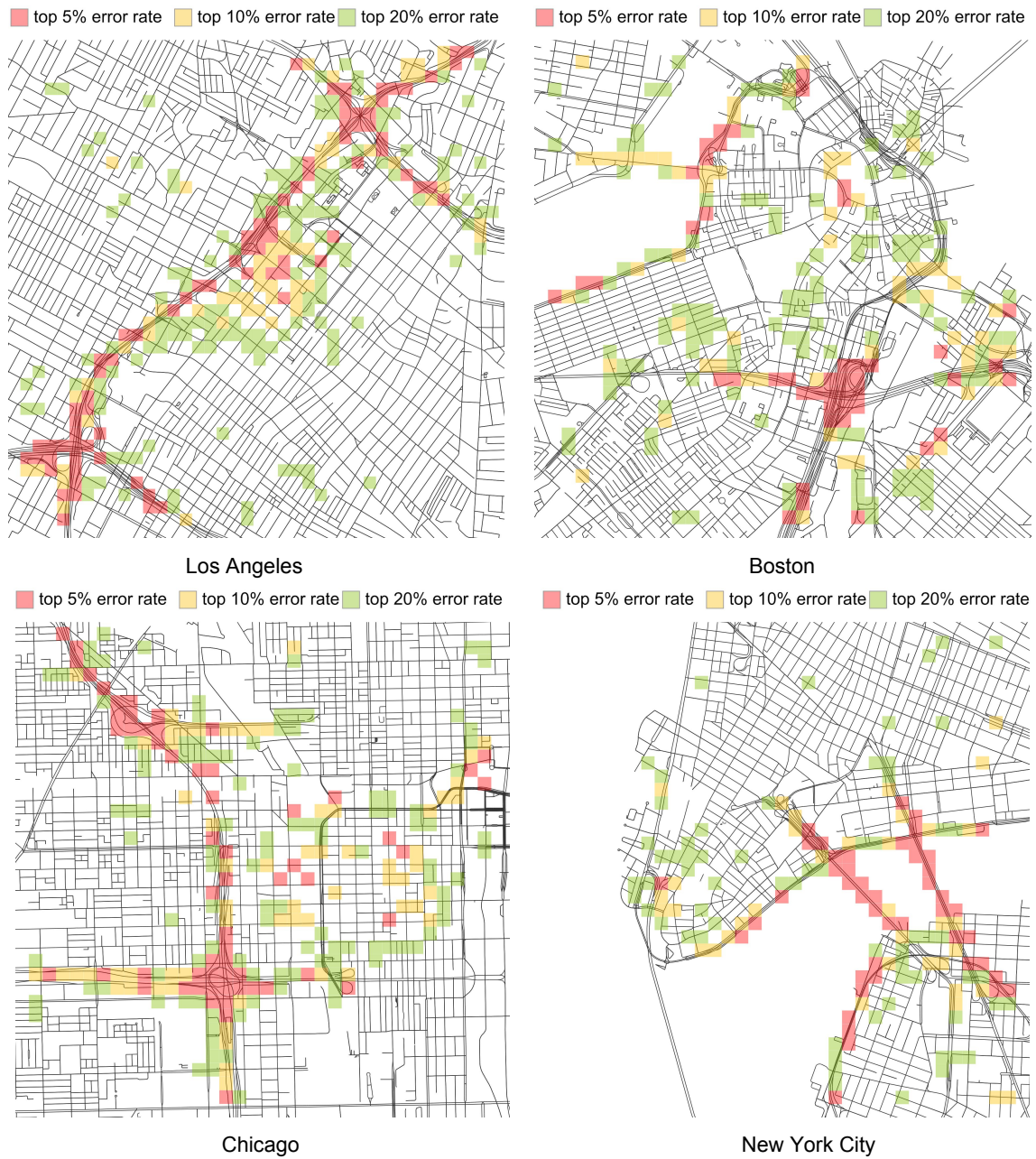
Figure 2-11: The distribution of the areas where existing schemes failed to infer the road network correctly.
