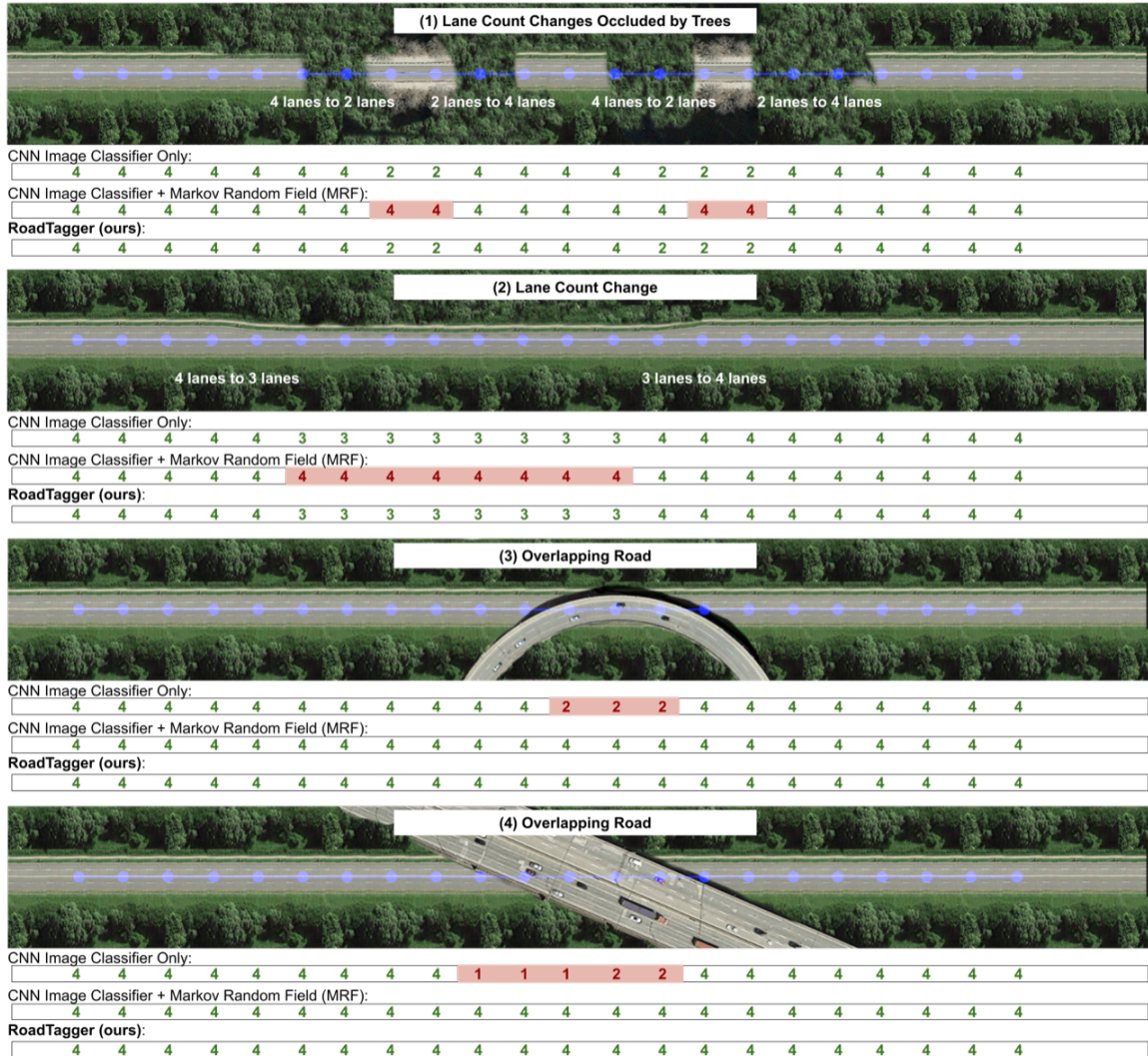
Figure A-1: Examples (1) to (4). In each image, blue lines show the road graph. The number of lanes predicted by the CNN Image Classifier, CNN image classifier with MRF post-processing and RoadAnnotator on each segment are shown along the bottom of each figure. We color the output numbers green for correct predictions and red for incorrect predictions.
