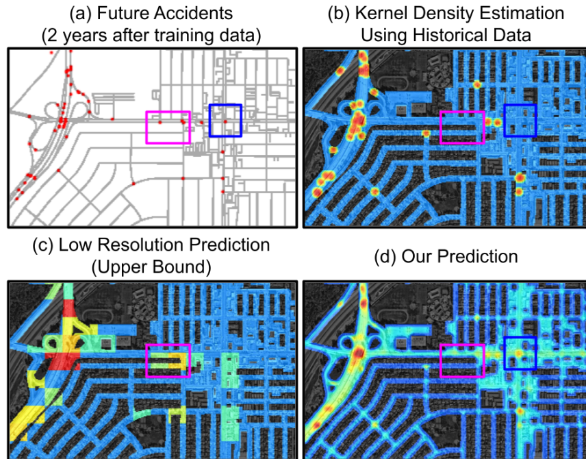
Figure 6-2: (b) Kernel density estimation (KDE) generally highlights areas with historical accidents as hot-spots. Therefore, it fails to predict new accidents (compare the blue box) and can only work for high-risk areas. (c) Low-resolution models have a high bias because they may assign the same risk score to a freeway and its neighboring residential road simultaneously (compare the purple box). (d) Our approach can identify high-risk locations that have not experienced accidents in historical data but are likely to experience accidents in the future. Note that the KDE predicts very specific risky locations, many of which do not have accidents in the future. In contrast, our method accurately highlights the roads where future accidents happen, properly attributing more risk to intersections and ramps. We did not visualize historical accidents as they look similar to KDE.
