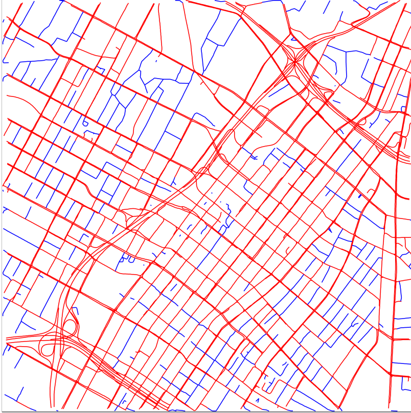
Figure 2-7: The merge result of RoadRunner (in red color) and an KDE based solution (in blue color) in Los Angeles
