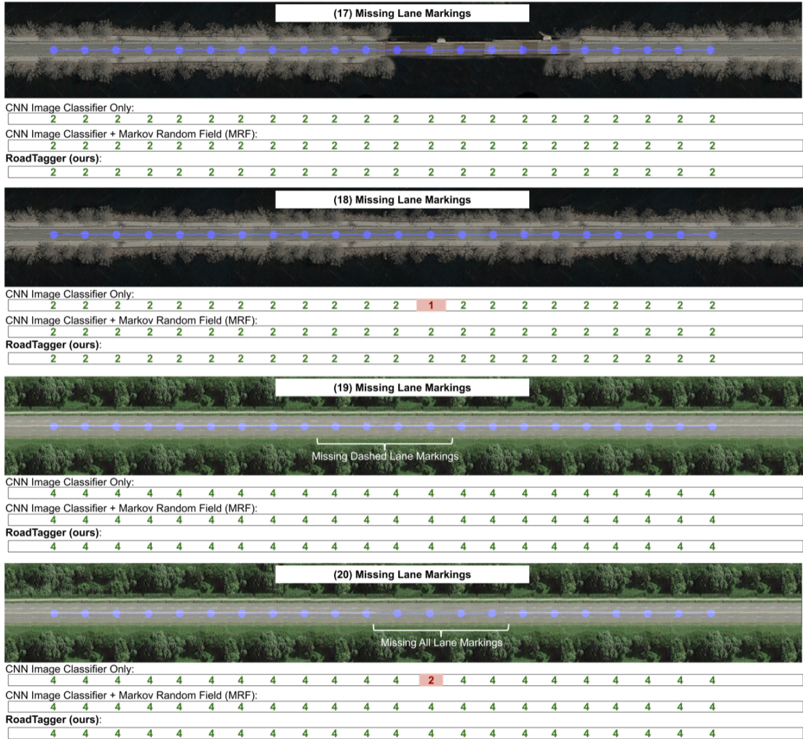
Figure A-5: Examples (17) to (20). In each image, blue lines show the road graph. The number of lanes predicted by the CNN Image Classifier, CNN image classifier with MRF post-processing and RoadAnnotator on each segment are shown along the bottom of each figure. We color the output numbers green for correct predictions and red for incorrect predictions.
