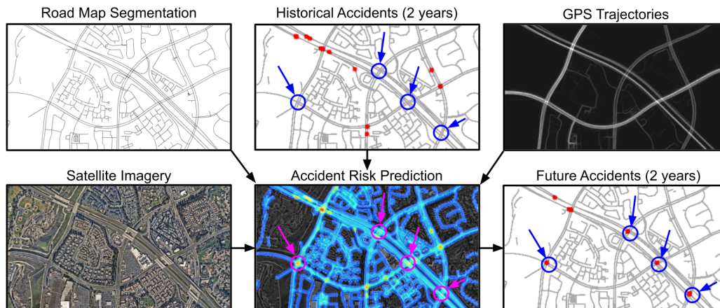
Figure 6-1: Our model inputs road maps, satellite imagery, GPS trajectories, and historical traffic accidents. It outputs accident probability distribution. Note that our model has identified a few locations as high-risk (highlighted with circles) even though they have no historical accidents. Locations that our model has identified as high-risk experienced accidents during the follow-up years.
