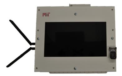
Figure 5-1: Upgraded AIO box with internal wireless capabilities
