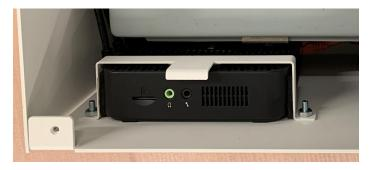
Figure B-27: GK41 mounted with bracket.
