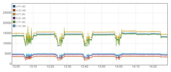
Figure 4-14: Potential icebreaking operations from NILM power stream.
