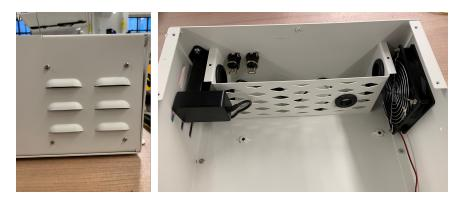
Figure B-15: Cooling fan installation (internal & external views).
