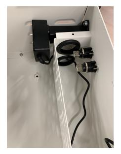
Figure B-12: UPS power cable wiring.
