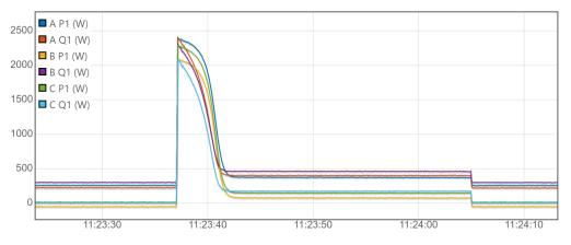
Figure 3-8: #1 MPDE Crankcase Blower on/off transient.
