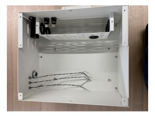
Figure B-8: Braided Conxall receptacle wires.
