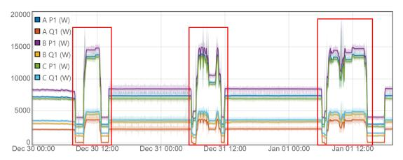
Figure 4-7: Multiple day measurement of panel 1-66-2 (underway periods highlighted).
