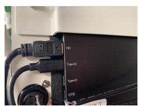
Figure B-36: WIMAXIT touch screen cable connection points.
