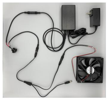
Figure B-24: Power cable configuration for AIO box.
