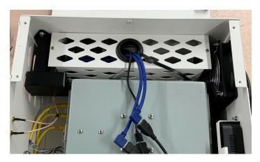
Figure B-21: Secured squirrel cage with appropriate cables exiting from the top opening.
