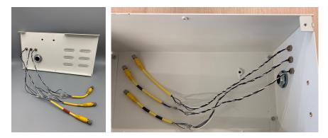
Figure B-10: Conxall cables attached to side plate #2.
