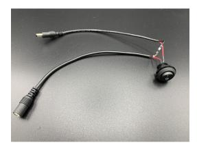
Figure B-29: Rocker switch with soldered wires.
