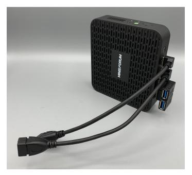
Figure B-23: GK41 with up/down USB adapters connected.
