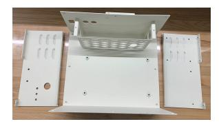
Figure B-4: AIO box with new side plates (expanded view).
