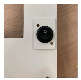
(b) Rocker switch inserted in adaptor piece.
