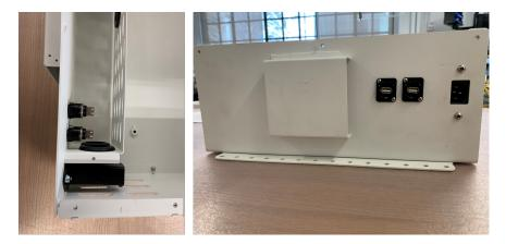
Figure B-11: Installation of USB-A panel mounts and IEC panel mount.
