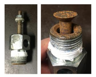
Figure 5-19: Deteriorated vacuum relief valve.
