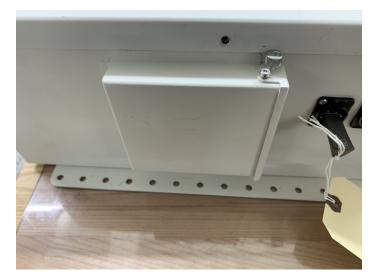
Figure B-35: Installed flip cover for external hard drive holder.
