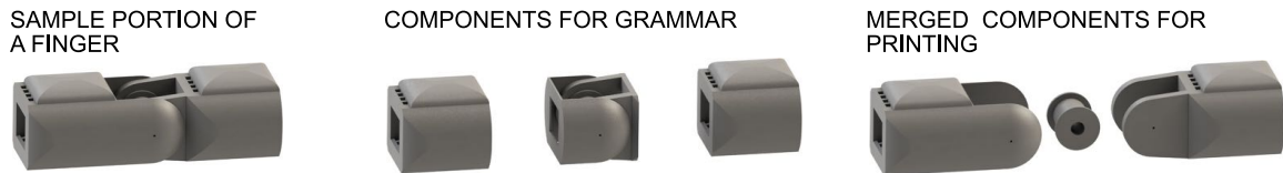
Figure 3-6: Grammar components correspond to mechanical systems rather than physical parts. They can be combined into their proper physical parts that are suitable for 3D printing after deformation.
