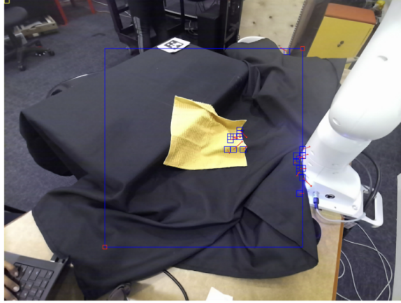
Figure 5-8: A view of the system attempting to pick the corner of a piece of cloth. The blue box indicates the cropped region of the image that is downsized and given as input to the hybrid controller’s models. The outputs of the controller are marked by small blue squares with red vectors to indicate the intended displacement.
