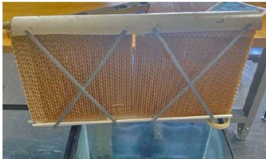
FIGURE 11: Testing Harness with Evaporative Cooling Pads in an Aquarium Test
