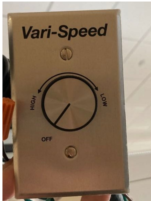
FIGURE 21: Fan's Control Switch
