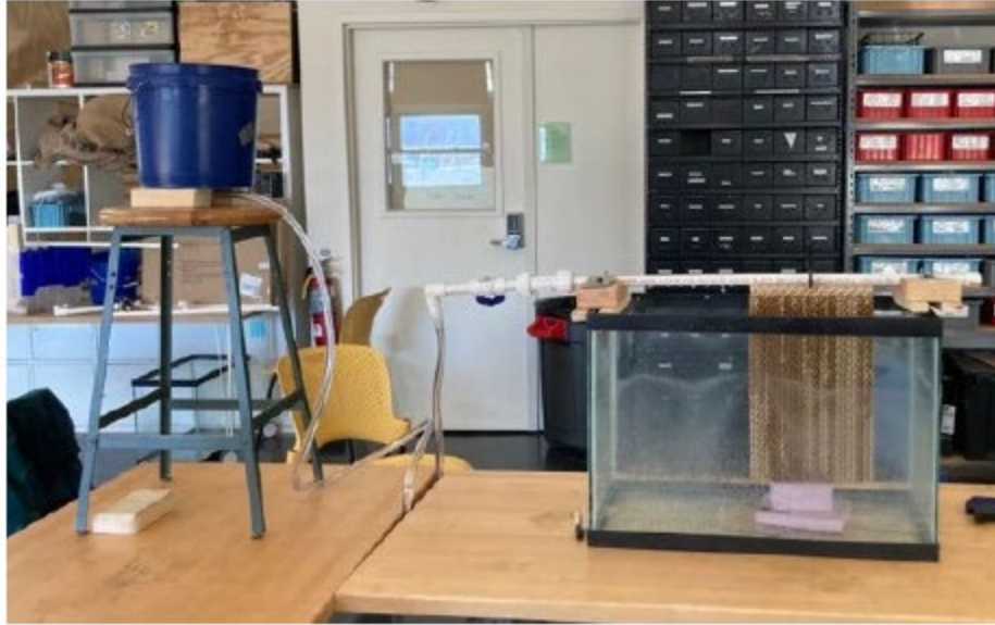
FIGURE 10: Aquarium Testing for Water Flow Rate
