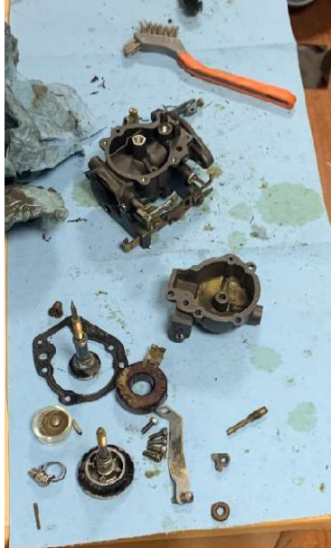
Figure 8: This image shows the carburetor partially disassembled. Varnish is clearly visible inside of the carb fuel bowl and the cork float is partially dissolved.
