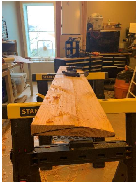
Figure 17: The aft foil during the shaping process. The outline of the foil cross section can be seen on the end of the board.
