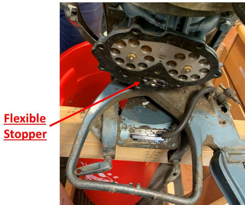
Figure 10: The rubber stopper can be seen here covering both pressure holes. This part was entirely removed from the engine.
