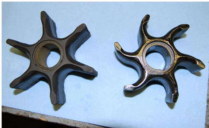
Figure 9: Side by side comparison of the old water impellor on the right and the replacement impellor on the left. Made from flexible plastic for optimum pumping, the impellers harden over time reducing their efficiency. An arm on the old impellor broke off shortly after removal from the engine.
