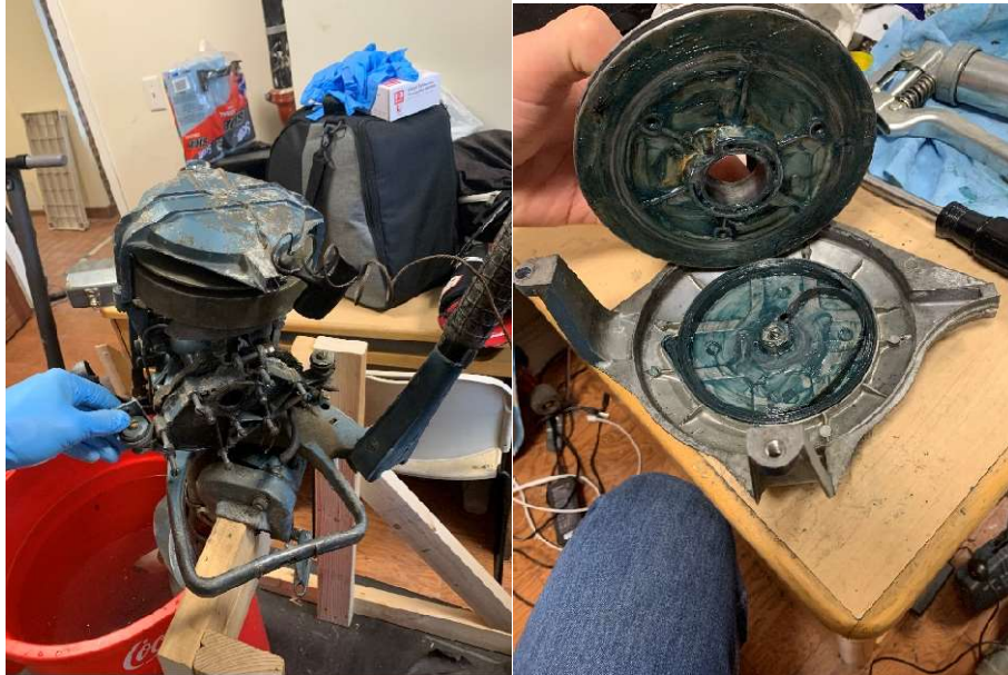
Figure 5: Left picture shows the frayed pull starting rope before disassembly. The right-hand picture shows the pull starter recoil spring installed inside its hubs. The spring had to be pretensioned to fit inside the housing and then generously coated in marine grease to reduce friction.
