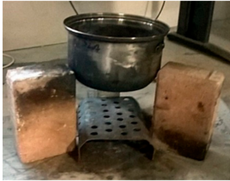
Figure 2-2: A grate insert known as the Mewar Angithi has been shown to improve the performance of three-stone fires [37].
