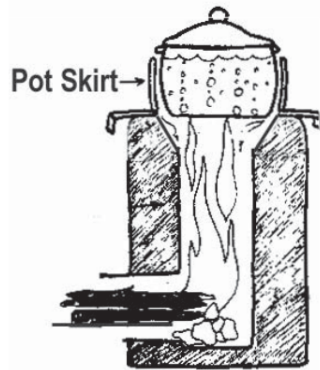
Figure 2-4: A pot skirt can keep rising hot gases close to the cooking vessel [35].
