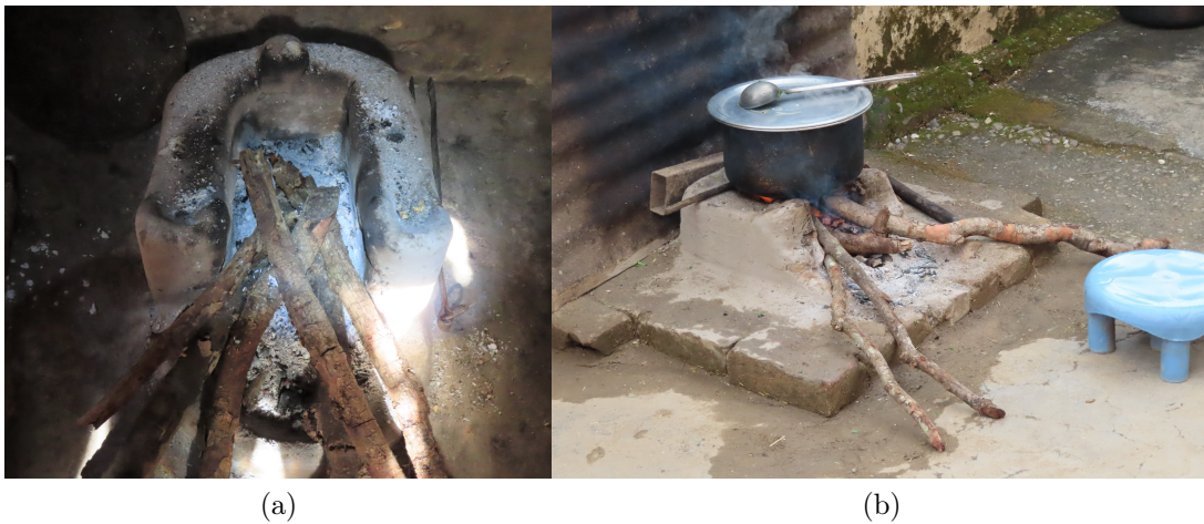
Figure 4-11: The indoor (a) and outdoor (b) traditional clay stoves in a Dehradun household.
