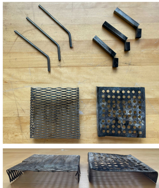
Figure 3-4: The prototype (left) and final (right) versions of the grate and pot stands tested on the D-Lab model stove.
