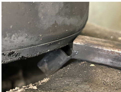
Figure 3-6: A cooking pot resting on the notch cut into the final design of the pot stands.
