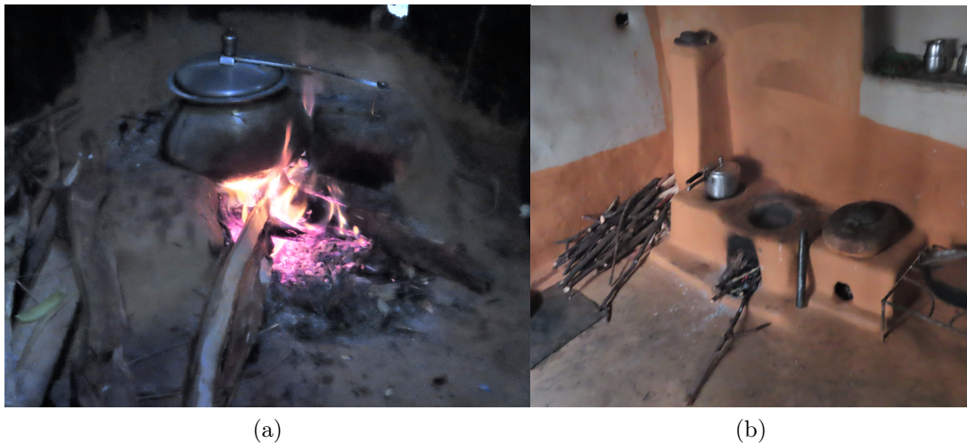
Figure 4-8: A traditional clay cookstove, built into the wall of the kitchen (a), and a professionally built improved cookstove (b) in Salambu.
