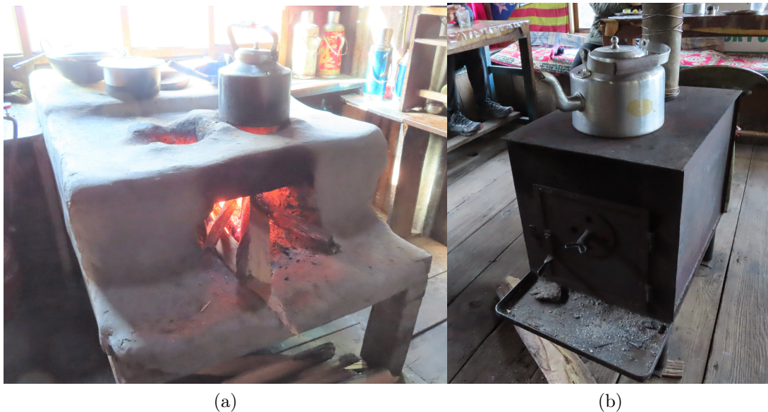
Figure 4-6: A typical large clay guest house cookstove (a) and a common metallic heating stove found at guest houses (b) in the Langtang Valley. A pot of water is warming on top of the heating stove.
