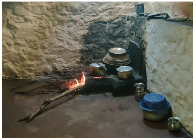
Figure 4-12: A three-pot clay stove in Chakrata operated with firewood. The D-lab model cookstove was based on the design of Chakrata stoves.
